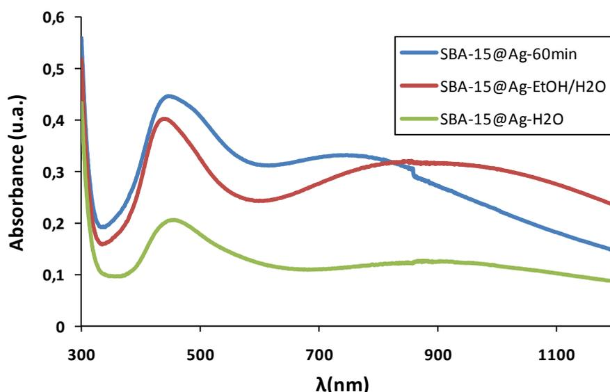
**Figure 48** Spectres UV visible des films : SBA-15@Ag-60 min, SBA-15@Ag-EtOH/H<sub>2</sub>O et SBA-15@Ag-H<sub>2</sub>O.
