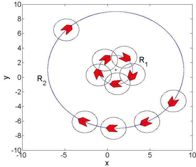
Figure 2.21: *Simulation of five agents governed by the control law from Corollary 2.4 which converge to a circular formation tracking a time-varying radius. The black circles represent the communication region of the agents. The figure displays two snapshots corresponding to different instants, at  $t = 20s$  the uniform distribution is not achieved yet and at  $t = 85s$  the splay state formation is stabilized.*
