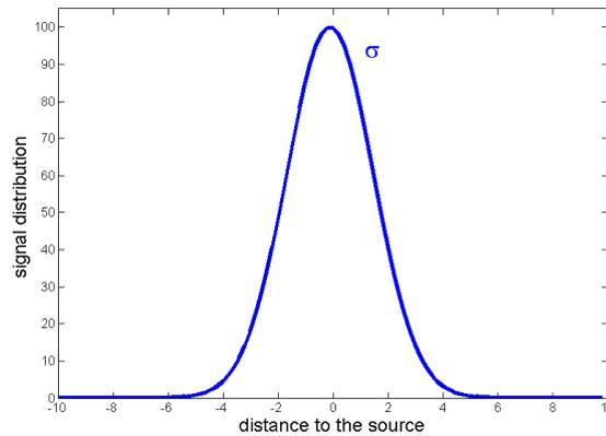
Figure 4.2: *Signal distribution modeled as a Gaussian function emitted by a single source.*
