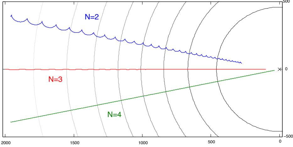
Figure 4.5: Trajectories of the formation center  $\mathbf{c}$  for different numbers of agents  $N$  when  $\sigma$  has circular level sets. Location of source is denoted by the  $\times$ . Image courtesy of Brandon J. Moore.
