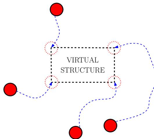
Figure 1.7: *Illustration of the virtual structure method*
