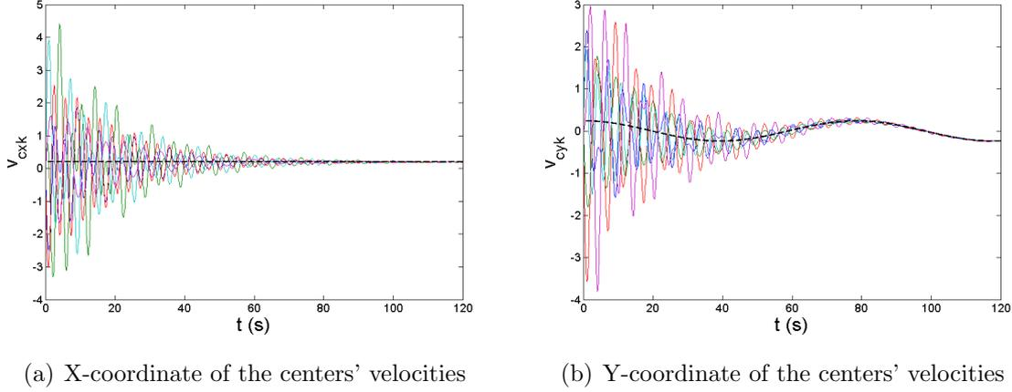
Figure 3.10: Evolution of the centers' velocities  $\mathbf{v}_{ck} = (v_{cxk}, v_{cyk})^T$  corresponding to the previous simulation of five agents shown in Figure 3.8 and the reference velocity  $\mathbf{v}_c^{ref} = (v_{cx}^{ref}, v_{cy}^{ref})^T$  (black dashed line).
