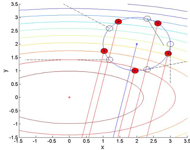
Figure 4.10: *Simulation of the distributed algorithm (4.33) by a circular formation of five agents centered at  $\mathbf{c} = (2, 2)^T$ . The function  $\sigma$  representing the signal propagation centered at the origin has elliptical level sets.*
