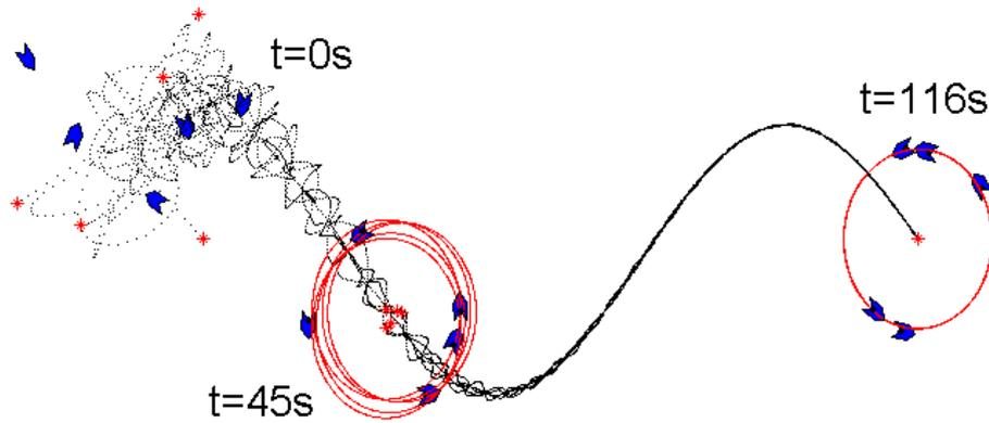
Figure 3.8: *Simulation of five agents governed by the control law (3.24) where the center computed by each agent results from the consensus algorithm (3.21). The black lines represent the centers' trajectories.*
