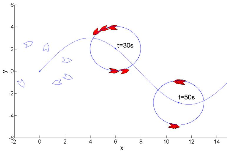
Figure 2.17: *Simulation of six agents governed by the control law from Corollary 2.1 with circular communication graph, tracking the reference of the center formation in blue. The figure displays three snapshots: the void blue agents correspond to the initial conditions and the red ones to two different instants, at  $t = 30s$  and at  $t = 50s$ .*
