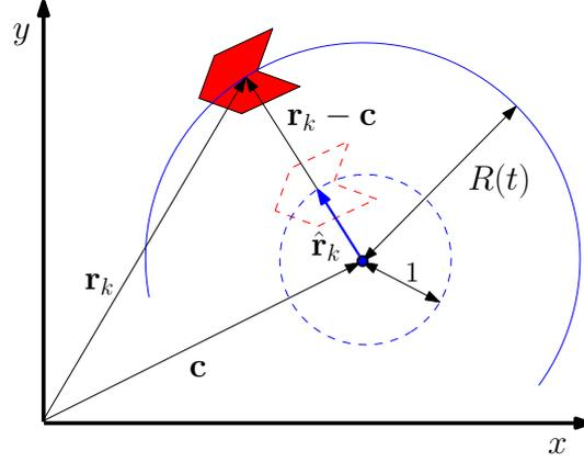
Figure 2.10: *Coordinates transformation for the scaling problem*
