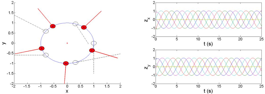
(a) Estimated directions  $\mathbf{z}_k$  for  $t = 0$ s (black dashed lines) and for  $t = 50$ s (red lines) (b) X and Y coordinates of estimated directions  $\mathbf{z}_k$
