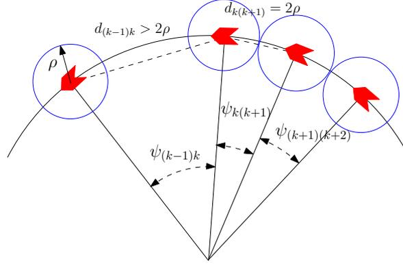
Figure 2.16: *Formation of communication chains during the contraction motion*
