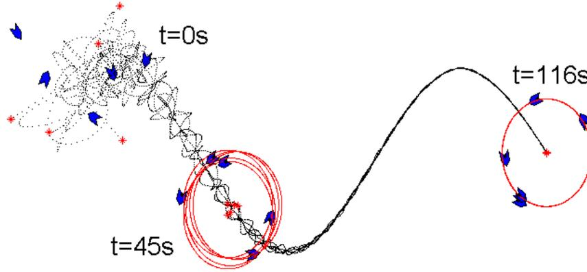
Figure 3.11: *Simulation of five agents governed by the control law (3.24) where the center computed by each agent results from the consensus algorithm (3.25). The black lines represent the centers' trajectories.*
