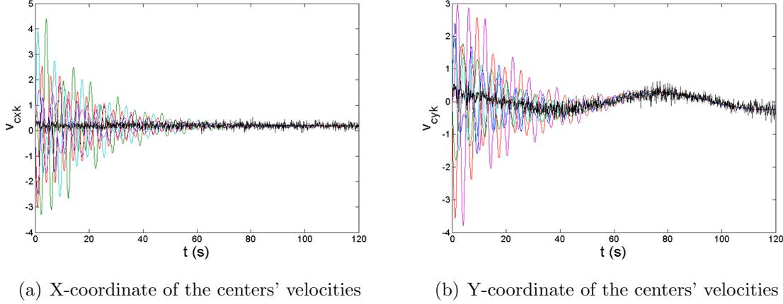
Figure 3.13: Evolution of the centers' velocities  $\mathbf{v}_{ck} = (v_{cxk}, v_{cyk})^T$  corresponding to the previous simulation of five agents shown in Figure 3.11 and the reference velocity  $\mathbf{v}_c^{ref} = (v_{cx}^{ref}, v_{cy}^{ref})^T$  corrupted by noise.
