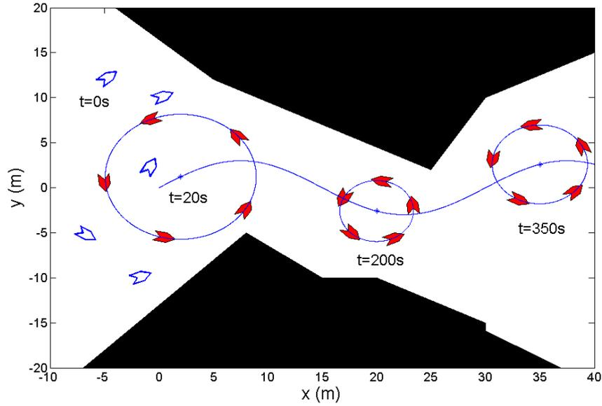
Figure 3.5: *Simulation of five agents governed by the control law (3.13) with  $\mathbf{G}(t) = \mathbf{T}_{c(t)} \mathbf{S}_{R(t)}$ . The circular formation, whose center tracks a time-varying reference, changes its radius in order to avoid the obstacles (black blocks).*
