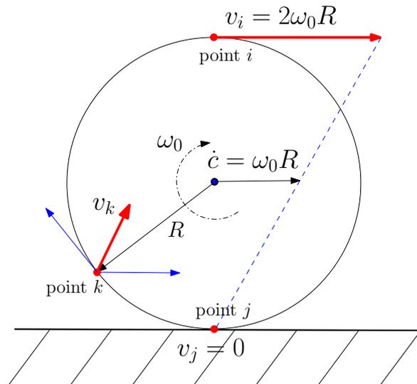
Figure 2.4: A wheel, rolling without slipping, with the velocity of three points shown
