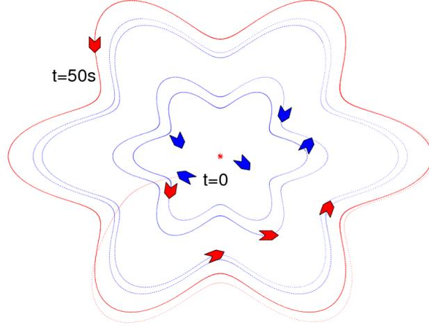
Figure 3.15: Simulation of five agents governed by the control law (3.34) and the reference of the radius  $R_k = \cos 6\alpha_k + 5$ . The red line represents the trajectory of one agent and the blue ones represent the final curves achieved for each agent. The figure shows two snapshots. The blue agents represent the initial conditions. The red ones represent the final state  $t = 50s$ .
