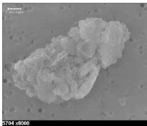
Fig. 8D.7c : SEM photograph of a coarse aggregate found in EDC sample #5704 (3137 m depth).
