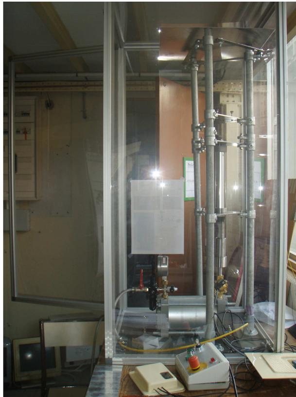
**Figure 5.3:** Air gun impact set-up from the laboratory *Mécasurf*. Laser barriers are not assembled on the photography.
