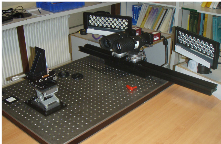
Figure 5.2: Stereo correlation set-up - Sample holding and positioning system, lenses, cameras and LEDs racks.
