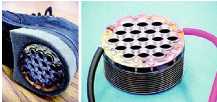
Figure 1.20 Dielectric elastomer heel strike generator. [69]
