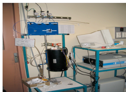
Fig 19 (b) Membrane calcination and reduction
