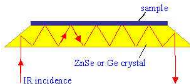
Principle of the HATR technique
