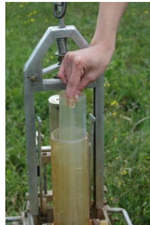
CAROTTIER MULTIPLE JENKIN-MORTIMER
