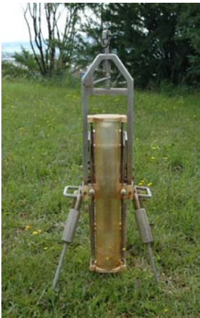
CAROTTIER MULTIPLE JENKIN-MORTIMER
