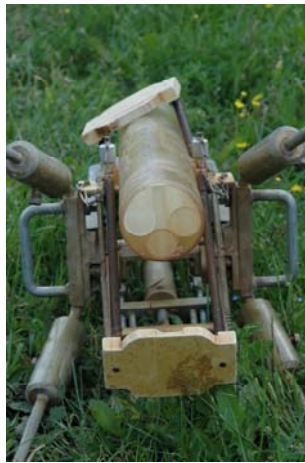
CAROTTIER MULTIPLE JENKIN-MORTIMER
