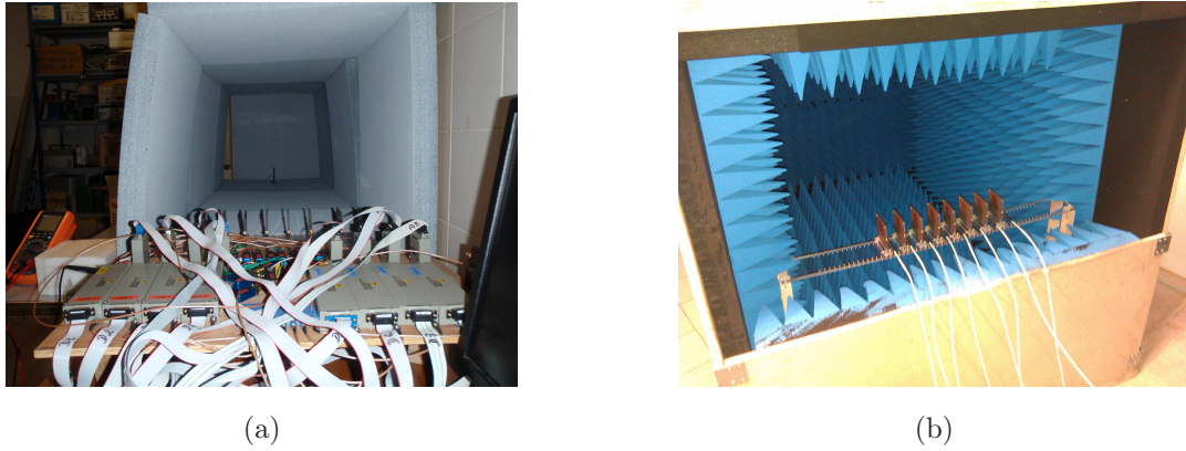
FIGURE 1.4: Photographs of the anechoic chambers built at LSEET with (a) flat and (b) pyramidal absorbing panels.
