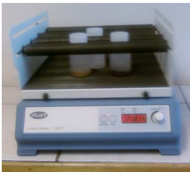
Figure A-5-2. Table de lixiviation
