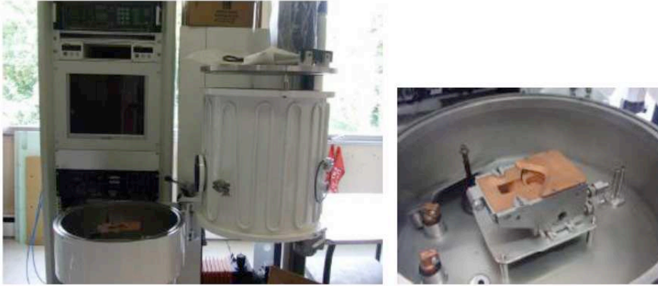
FIGURE 11.5: Picture of the aluminization facility in IPN Orsay used to evaporate a layer of 200 nm of ultra radiopure aluminium on the entrance face of the BiPo-3 scintillators
