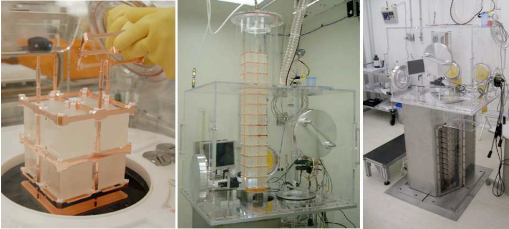
FIGURE 4.5: Pictures of the CUORE-0 tower during its assembly in LNGS.
