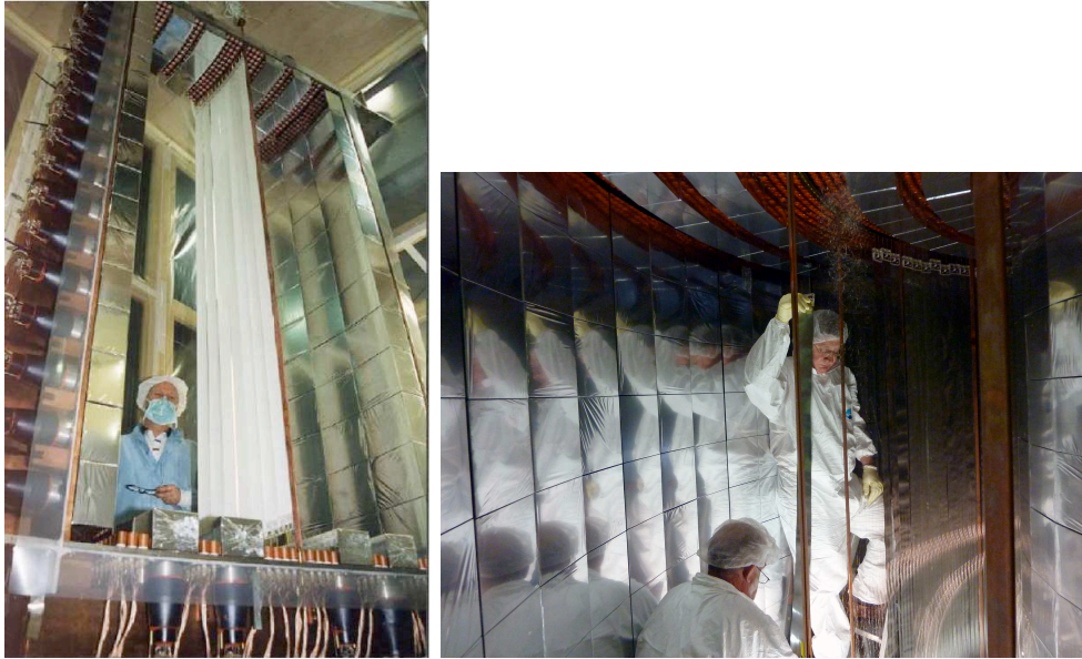
FIGURE 2.2: (Left) View of a sector inside the LSM clean room during the assembly of the source foil. Note the double beta foil strips (in white) and the copper calibration tube besides, the scintillator blocks wrapped with aluminized mylar, the PMT's in the back surrounding by black tubes and the copper rings on the top and bottom of the tracking Geiger cells (the wires are too thin to be seen here). (Right) view inside of the detector during the dismounting of the sources foils in April 2011.
