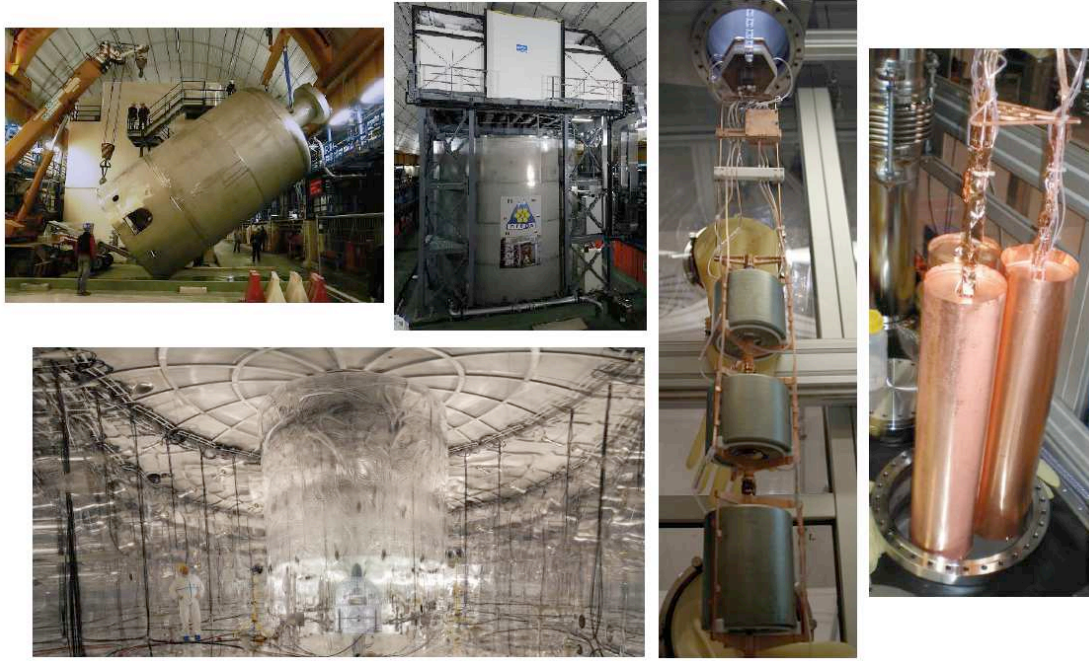
FIGURE 3.4: Some pictures of the GERDA assembly : the stainless steel cryostat ; the water tank and the clean room above ; inner view of the water tank ; deployment of the first array with three natural germanium detector ; deployment in November 2011 of the 3 arrays with 8 enriched germanium detectors (17.7 kg of ^{76}\text{Ge} , GERDA Phase 1).
