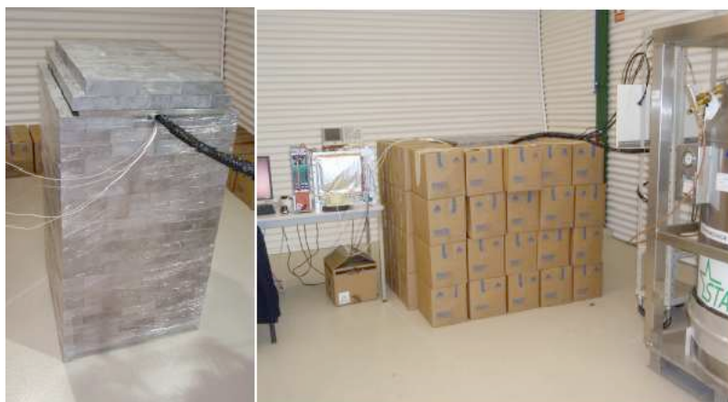
FIGURE 11.17: Pictures of two configurations of shield tested with the BiPo-3 prototype in Canfranc.
