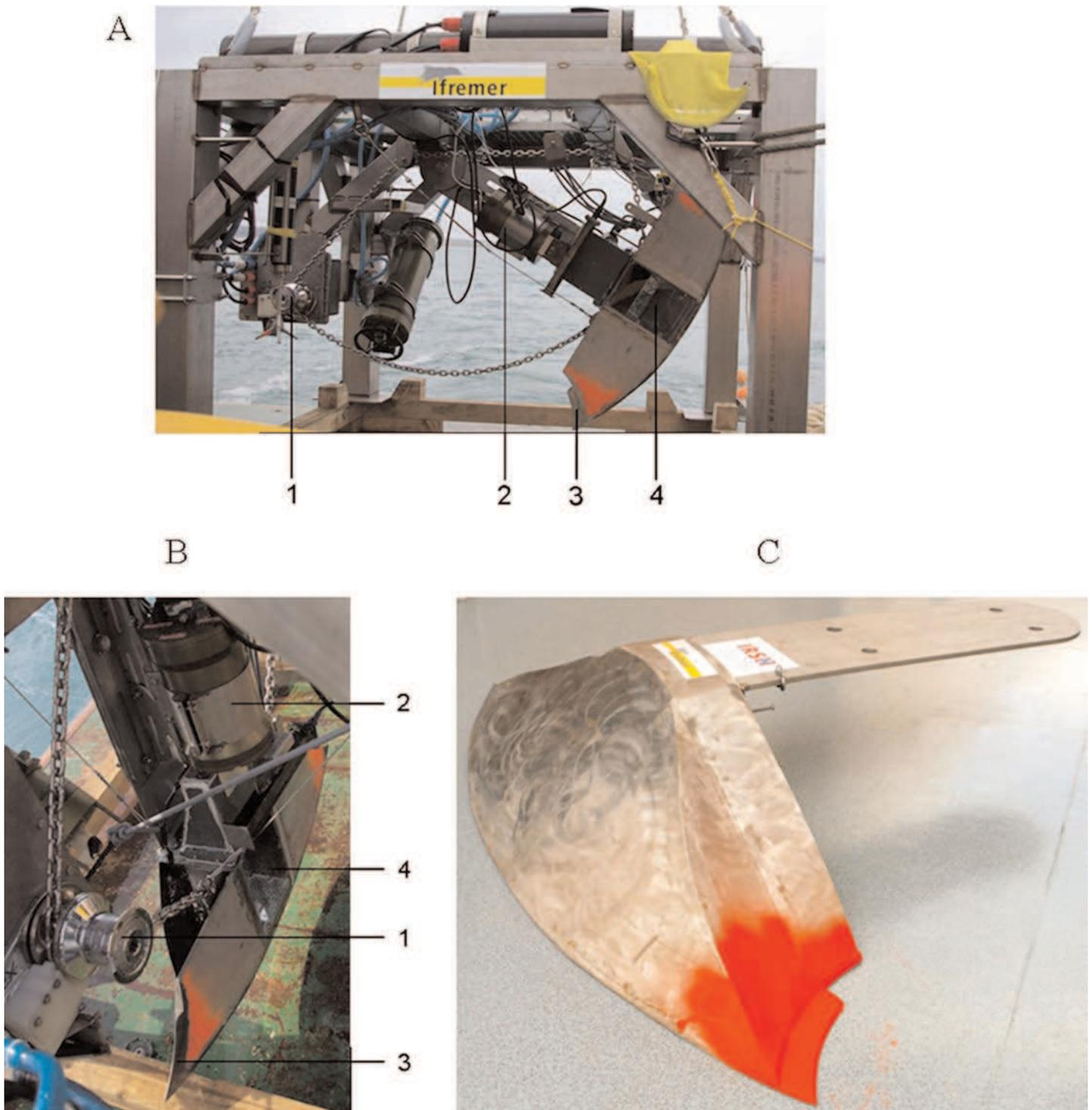
**Fig. 2.** Design of the walking beam. (A) General view of the beam mounted on its frame. (B) View from above: a strictly planar surface at the front, a cone section profile at the back. (C) Rear view. 1 = motorized winch, 2 = video camera housing, 3 = cutting blade, 4 = periscope box.
