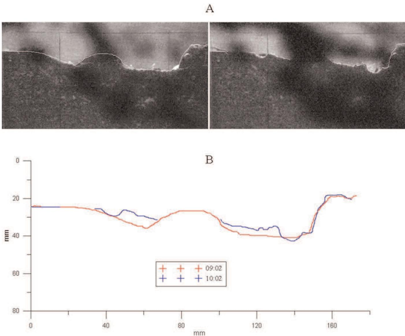
**Fig. 12.** (A) Images of the vertical section view at 09:02 (left) and 10:02 (right). Black clouds are particulate deposits covering the horizontal faceplate of the periscope box. (B) 2 interface levels corresponding to the images (A).
