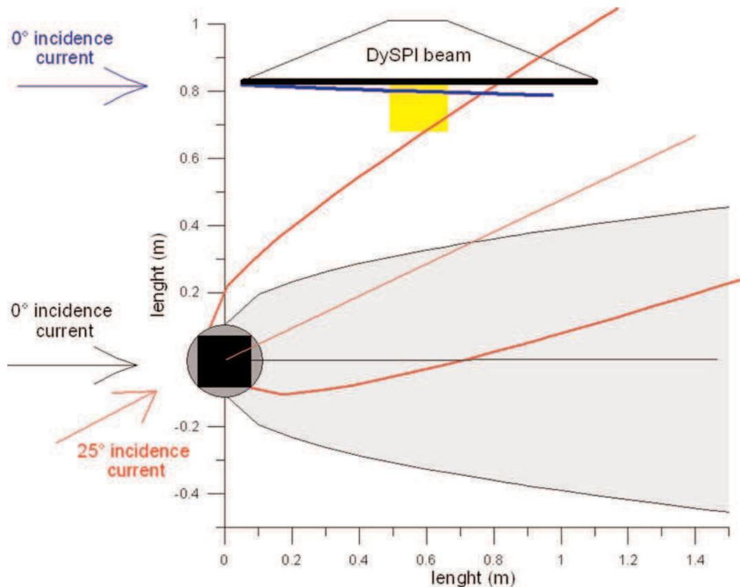
**Fig. 6.** Boundary layer thickness (blue) for a zero degree incidence current and foot wake pattern when DySPI is positioned right in the current direction (gray) and for a current –beam angle of 25° (red). The observation area (yellow) is impacted for this last angle.
