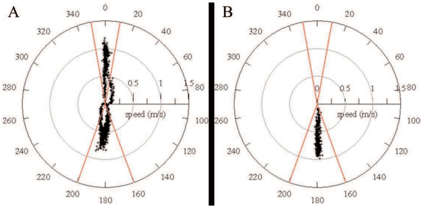
**Fig. 8.** Tidal current roses during 2 different deployment periods, measured 30 cm above bottom using an ADV. The 0°-180° axis is the beam axis. (A) DySPI has been deployed during a whole tidal cycle. (B) DySPI has been deployed during a whole ebb period. The frame was correctly positioned in the current direction.
