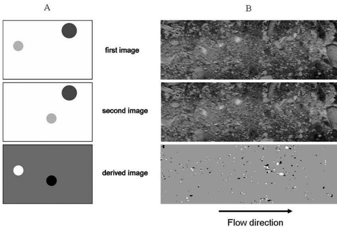
**Fig. 11.** Subtraction technique of two images to filter out non-moving particles. (A) Schematic illustration of the difference between two images with one moving and one nonmoving particle. (B) Application of the subtraction technique to images from DySPI acquired at 09:02. Time delay between these two images is 11/25 s, 0.45% of the surface has moved during this period.
