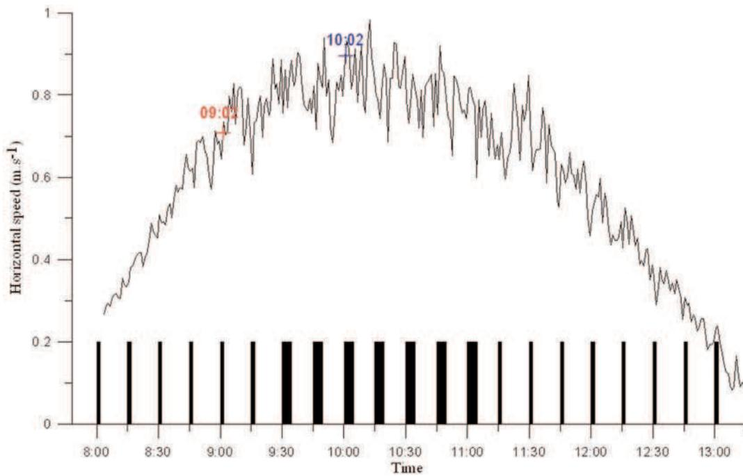
**Fig. 10.** Time series of horizontal velocity 30 cm above seabed (ADV) averaged every minute during the whole deployment period. Black bars represent video acquisition periods. The dates of image processing presented below (Fig. 11 and 12) have been highlighted.
