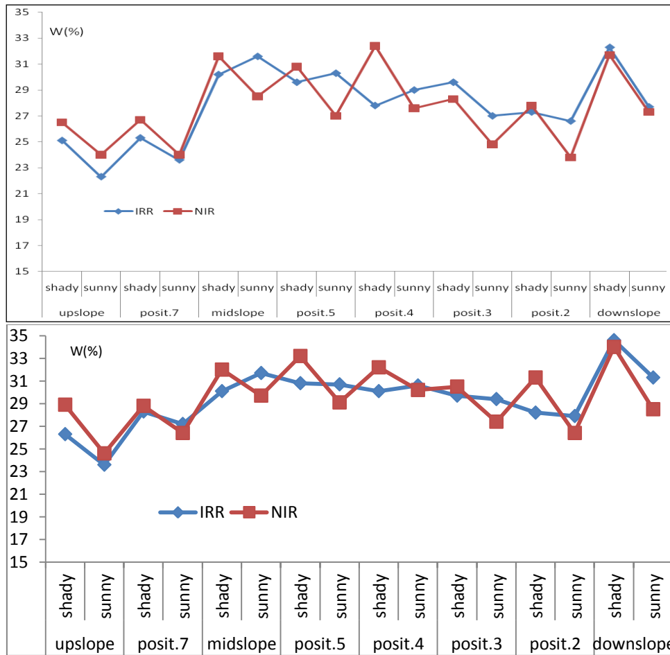
Fig. 3.29a & b: Distribution along the slope of gravimetric water content (W) in the upper soil layer (a) and in deeper soil layer (b), Gačnik, May 2005.
