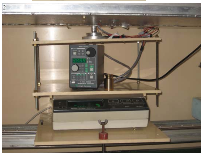
Fig.VI-1: Closure view photograph of the experimental arrangement (1) inside the wind tunnel, and (2) below the test chamber, temperature controller with electronic weight balance.
