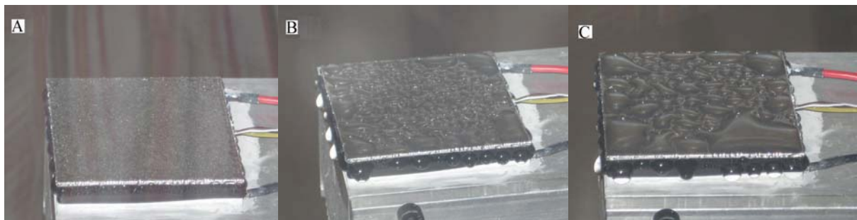
Fig.VI-3 : Photographs of flat plate showing the falling drops of condensate before applying sponge from the vertical surface of the plate (a) after 40 min of the exp (b) after 5 h and (c) after 7 h 30 min of the condensation exp (CEI-7).
