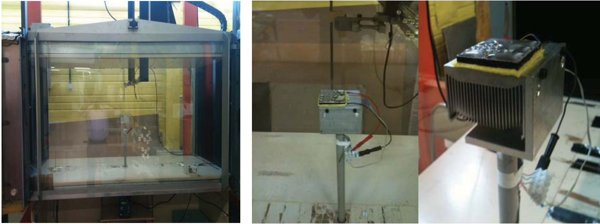
Fig.IV-2 : Photograph of test chamber and a closer look of condensing unit
