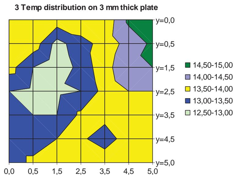
Fig.III-3: Temperature distribution experiment with a plate having a slight concavity.
