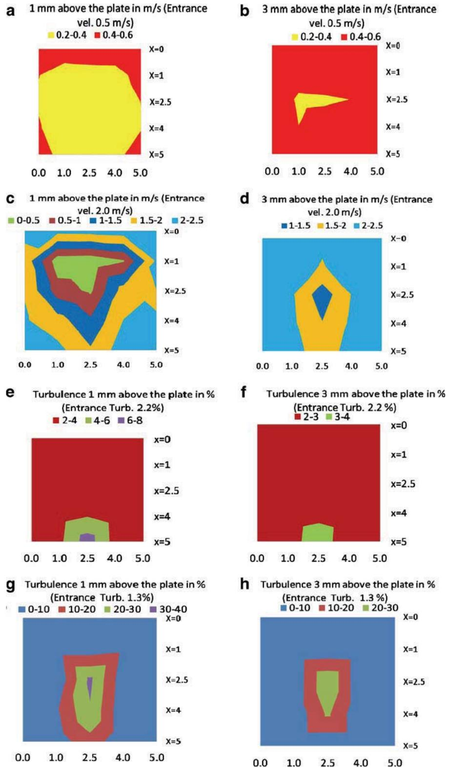
**Fig. 4 a–d** Comparative surface plots of a flat plate in vertical position (a, b) velocity profile in metre per second for (a) ambient temperature ( $T_a$ )=21.1°C and (b) at ( $T_a$ )=19.9°C (c–d) and turbulence intensity in per cent
