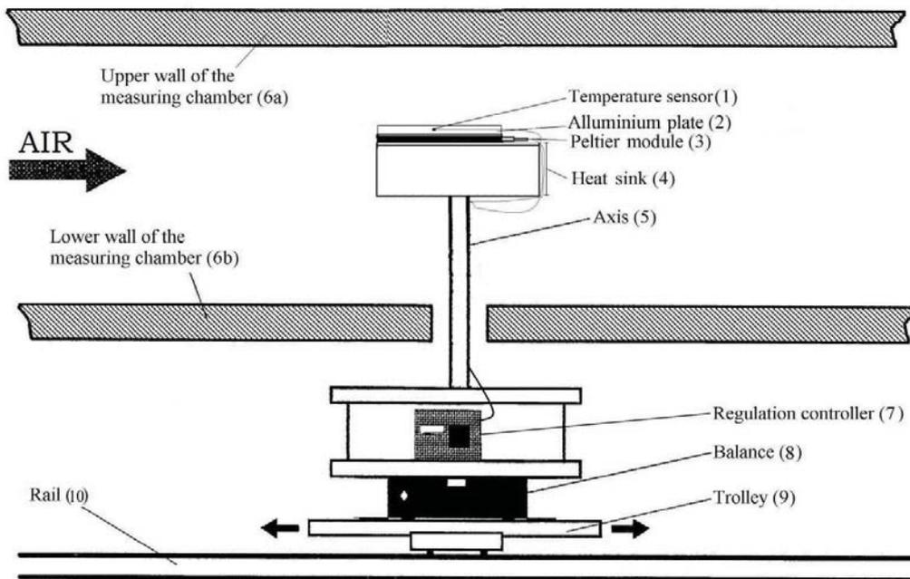
Figure 4. Schematic of the whole condensation unit.
