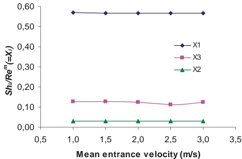
Fig.VI-21: Re-plotted data of figure VI-20, by using  $Sh_i/Re^{m_i}$  as ordinate and mean entrance velocity as abscissa.
