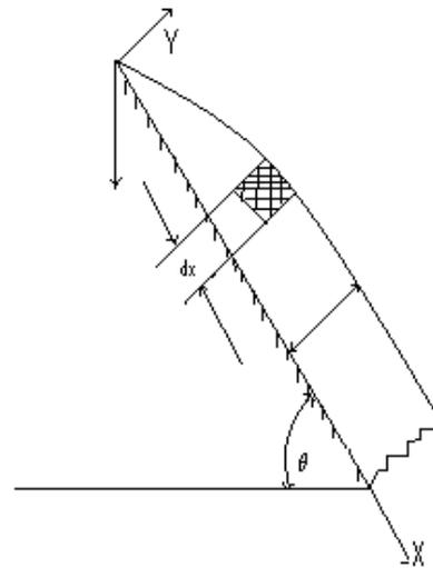
Fig.I-1: Flow of laminar film on a plate.
