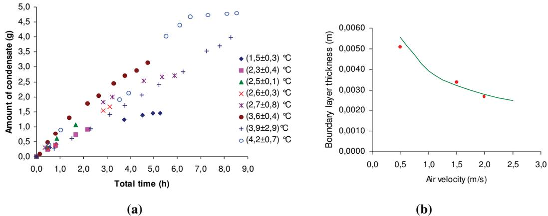
**Figure 5. (a) Amount of condensate as a function of total time of experiment for 8 experiments (b) Comparative plot of boundary layer thickness calculated by using Blasius solution (continuous line) and (observed experimentally) on a plate of surface area 5 cm x 5 cm.**
