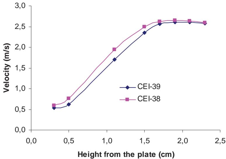
Fig.IV-15: Comparative plots of two experiments (CEI-38, CEI-39) showing variation of velocity at last middle point of the plate (i.e.  $X = 5.0$  cm,  $Y = 2.5$  cm,  $Z = 0.3 - 2.3$  cm) from inside the boundary layer to free flow stream.
