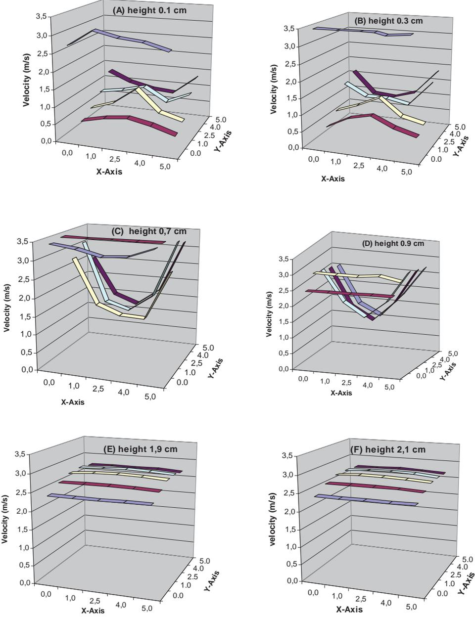
Fig.IV-16 (a, b, c, d, e, f): 3D curves of the velocity profile at fan frequency 32.1 Hz and mean entrance velocity 2.5 m/s at different heights from the surface of the plates. X and Y – Axis representing the plate cross section on which the velocity measurements have been taken. Z- Axis as velocity (m/s).
