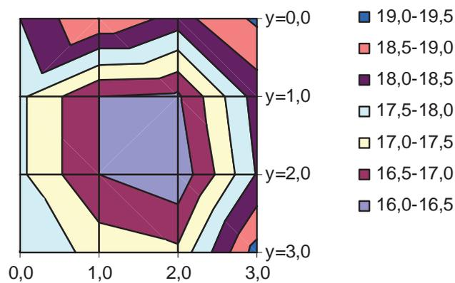
Fig.III-4: Temperature homogeneity plots on the surface of the ceramic plate of Peltier element on the cold side (without metal plate).
