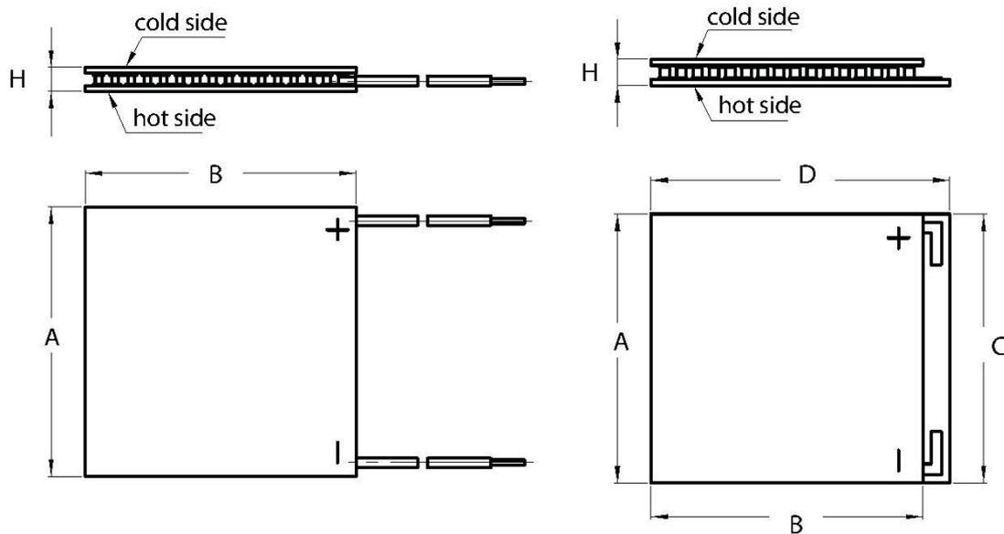
Fig.II-8: Sketch of the dimensions of Peltier element.
