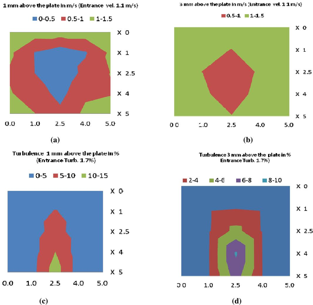
**Figure 3. (a-d) Comparative surface plots for the flat plate in horizontal position (a-b) velocity profiles in metre per second for ambient temperature 21.8°C and (c-d) turbulence intensity in per cent.**
