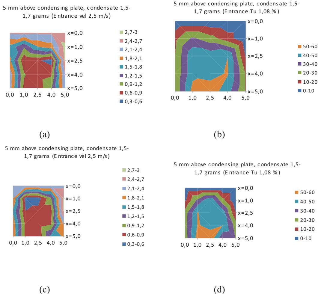
**Fig.IV-13 (a-d):** A comparative surface plots of (a, c) velocity profile (m/s) and (b, d) turbulence intensity (%) on a horizontal flat plate at 5 mm height during condensation on increasing weight (from 1.5 g to 1.7 g) of condensate on the surface of the plate for 2.5 m/s velocity in two different experiments- (a-b) CEI-38, and (c-d) CEI-39.
