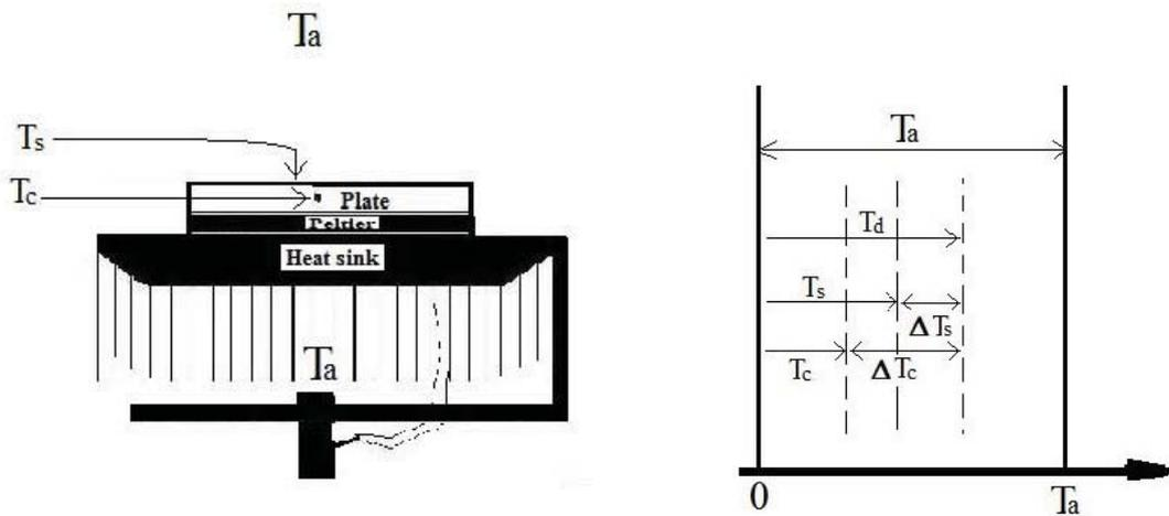
Fig.II-4: Representation of different temperature levels on the active condensing unit.
