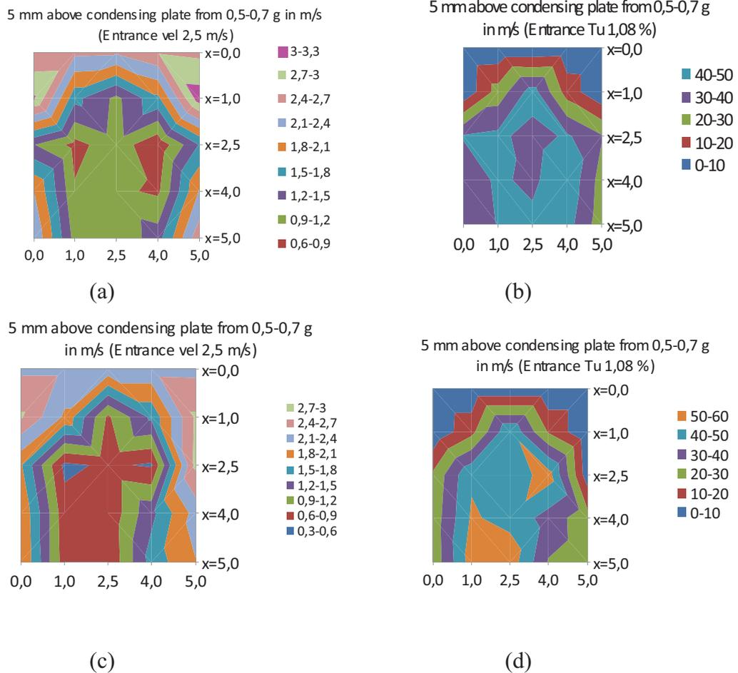
**Fig.IV-12 (a-d):** A comparative surface plots of (a, c) velocity profile (m/s) and (b, d) turbulence intensity (%) on a horizontal flat plate at 5 mm height during condensation on increasing weight (from 0.5 g to 0.7 g) of condensate on the surface of the plate for 2.5 m/s velocity in two different experiments- (a-b) CEI-37, and (c-d) CEI-39.
