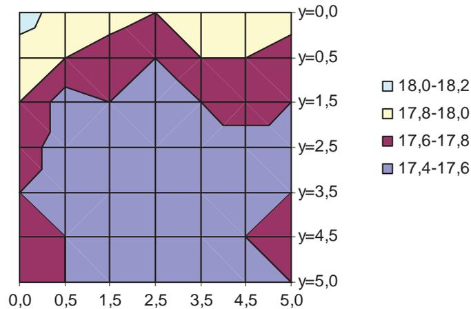
Fig.III-6: Distribution of surface temperature with a plate of 3 mm thickness.
