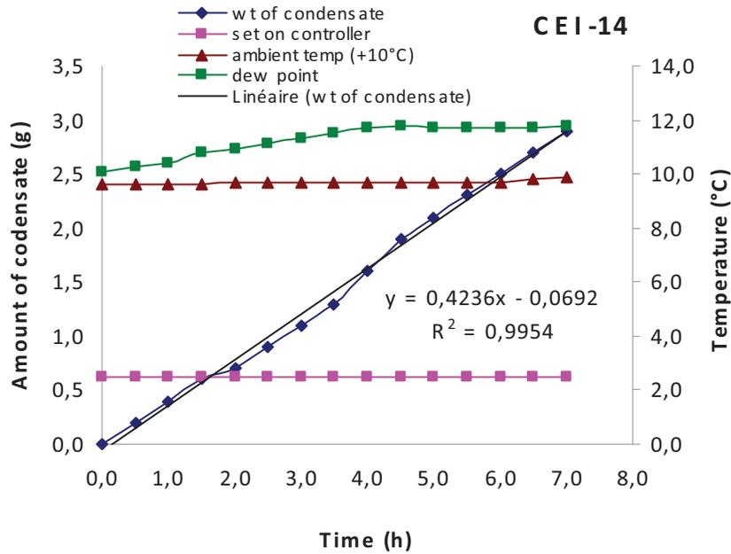
Fig.VI-4: Plot of amount of condensate and secondary Y-axis as temperature ambient (-10°C), dewpoint, and set on controller with respect to time.
