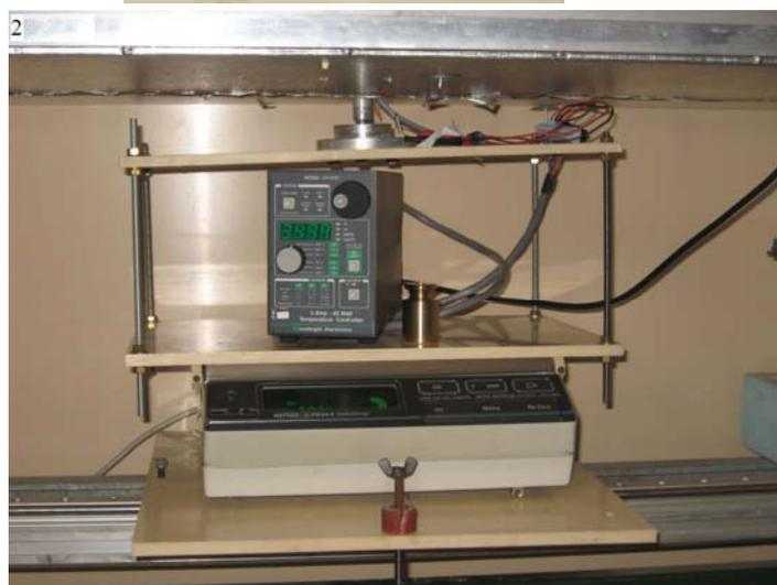
Fig.VI-1: Closure view photograph of the experimental arrangement (1) inside the wind tunnel, and (2) below the test chamber, temperature controller with electronic weight balance.
