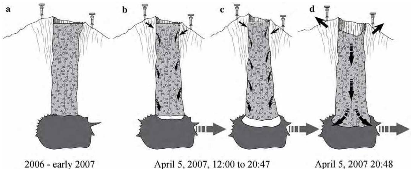
**Fig. 14.** Scenario of the Dolomieu caldera collapse. a) The rock column beneath Dolomieu crater is supported due to the pressure in the magma chamber. b–c) Rapid lateral withdraw of magma from the magma chamber lowers the pressure in the latter and deflate the summit of Piton de la Fournaise. d) The rock column collapses into the magma chamber relaxing the Piton de la Fournaise massif.
