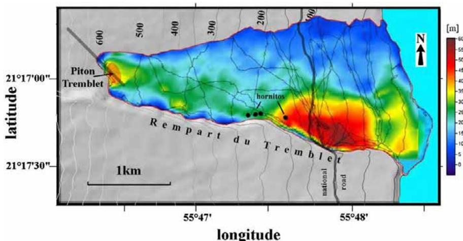
**Fig. 6.** The April 2007 lava flow. Shown are colour coded thickness of the lava flow, determined by cinematic GPS measurements and subtraction from a pre-existing DEM. Black curves represent the post-eruption GPS campaigns on the lava flow.
