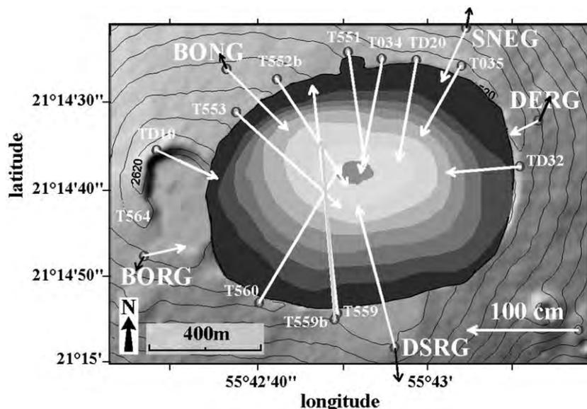
**Fig. 12.** Pre- and post-collapse ground displacements of the Piton de la Fournaise massif. Shown are the horizontal ground displacements as recorded by the permanent (large characters) and punctual GPS network (small characters). Black arrows represent pre-eruptive and pre-collapse expansion of the Dolomieu crater recorded by the permanent GPS network, while white arrows represent post-collapse inward motion of the crater from April 6 to end of November 2007.
