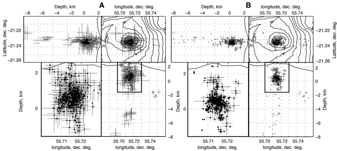
FIGURE 9.4 – Comparison between localizations and relocation
