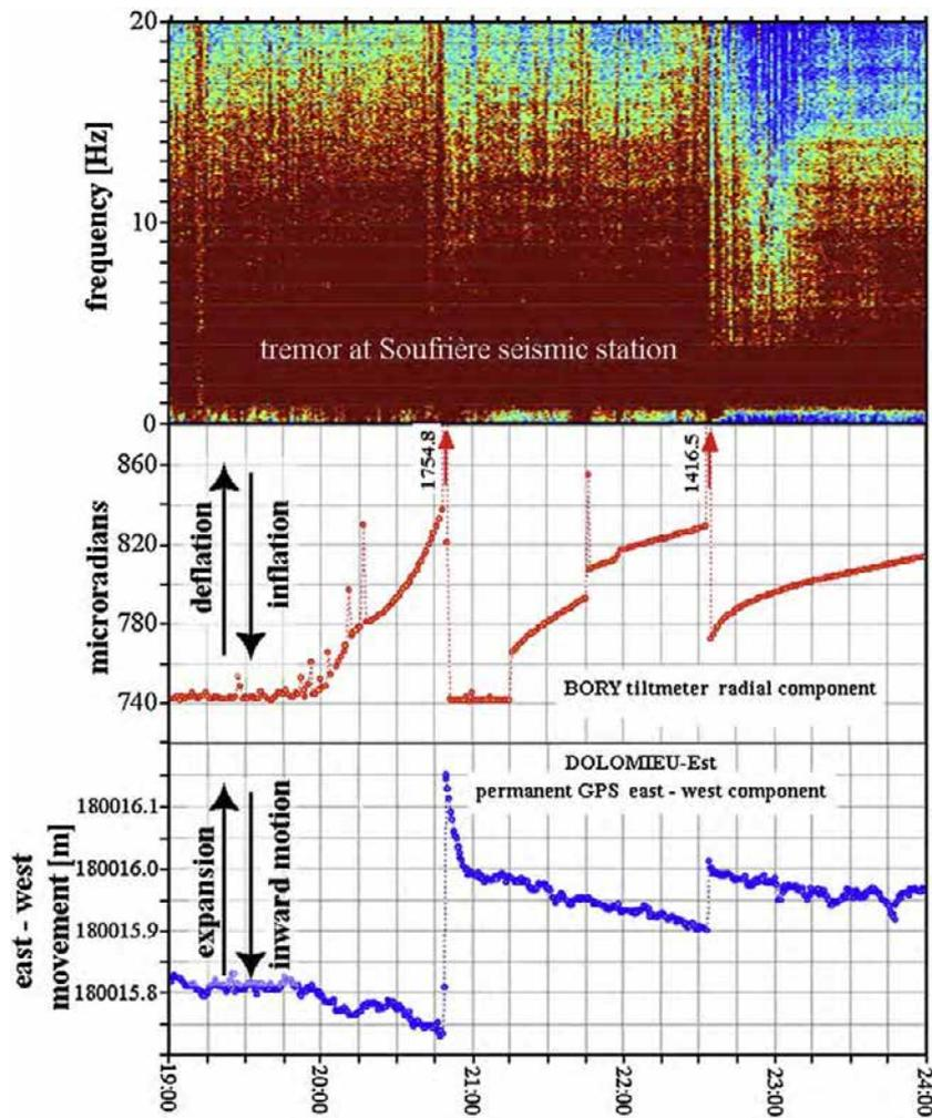
**Fig. 9.** Enlarged spectrogram and deformation plot. This representation covers of the period on April 5 between 19:00 and 24:00 revealing the close correlation between tremor recorded by the Soufrière seismic station, tilting and the Dolomieu-Est permanent GPS station. Note that the tiltmeter maximum values were out of range and the values are indicated in the plot.
