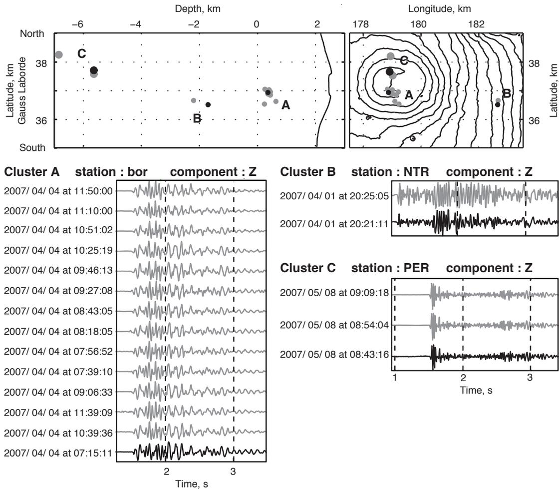
FIGURE 9.2 – Comparison between hand made localizations and waveforms. *Left : localizations. Right : waveforms. 3 clusters are represented, A : around sea level, B : under east side of Piton de la Fournaise volcano, and C : at -5 km. For each cluster, the black earthquake (black dot on map and blue signal) is the hand localized master (best constrained localization), the grey earthquakes represent the hand localized slaves (their corrected pick times are aligned on the master).*
