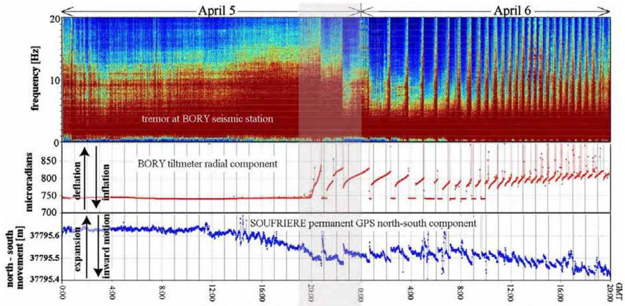
**Fig. 8.** Spectrogram and deformation plot of April 5 to April 6. Top: spectrogram of seismic tremor during April 5 and 6; middle: radial component of the Bory tiltmeter station; bottom: Soufrière permanent GPS North-South component. Note the close correlation between tremor intensity, tiltmeter and GPS movement starting on April 5 at 20:48 and lasting until early April 7. Greyish area corresponds to the time window shown in Fig. 9.
