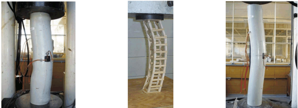
Figure 1.14 Examples of buckling in column [www civildb], [www highline]
