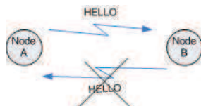
Figure 2.8: An asymmetric link from node A to B in OLSR
