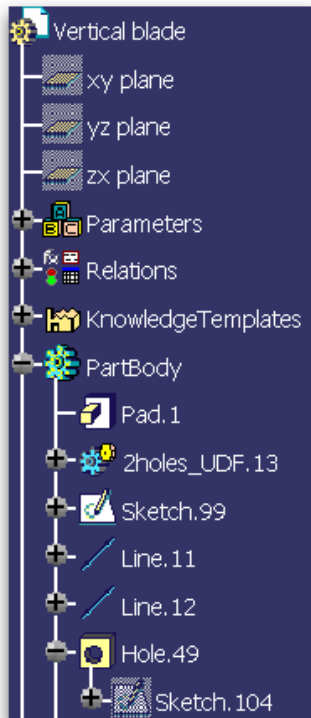
(a) CATIA V5's specification tree of the Vertical Blade part, presenting its aggregated elements.
