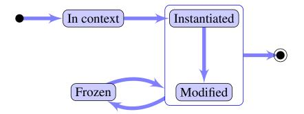
Figure 10.1 – Template instance status evolution during its life cycle.
