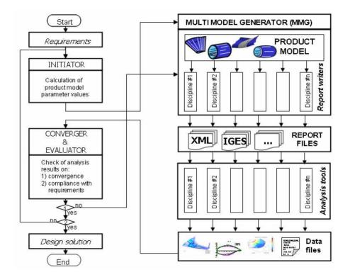
Figure 5.2 – Paradigm of the Design and Engineering Engine with the Multi-Model Generator [LA ROCCA AND VAN TOOREN, 2009].
