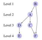
**Figure 4.5** – Four-level hierarchy resulting from the application of SUGIYAMA *et al.* [1981]'s graph layout algorithm on the graph presented in figure 4.2.
