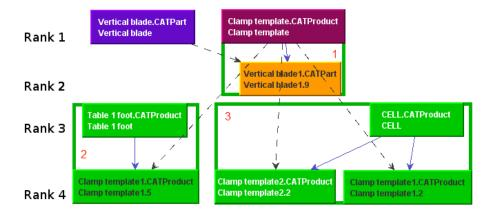
Figure 12.3 – Resulting update sequence with groups after the modification of two templates. Dashed arrows are *InstanceLocation* links (see section 9.2.6.1) and blue arrows are *Instance* links (see table 6.1, page 78). Rank 0 contains the modified documents. Ranks 1 to 3 contain the documents to update. Groups marked 1, 2 and 3 show documents that have to be checked-out together.
