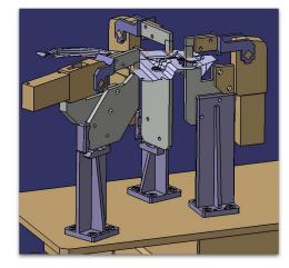
(b) Three template instances from the same template with various configurations holding a metal sheet
