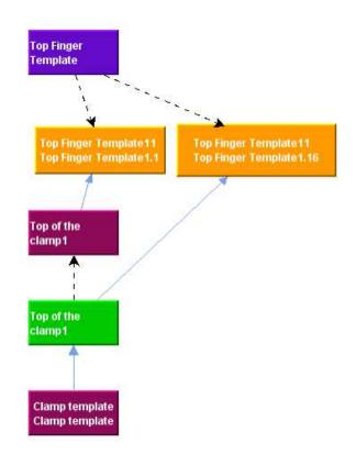
Figure 10.6 – Example of an indirect instance that has to be removed from the sequence as it will be overwritten by the containing template. Example taken from CATIA V5. Blue arrows show *Instance* links (see table 6.1, page 78) and black arrows *InstanceLocation* links (see section 9.2.6.1).
