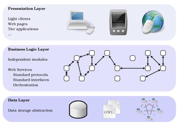
Figure D.1 – Schema representing a three-tier architecture.
