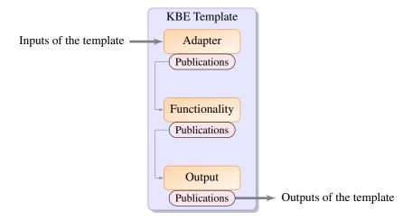
Figure 1.5 – Generic structure of a KBE template with data flow.
