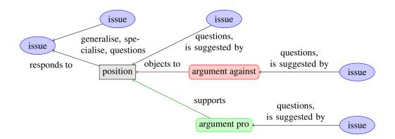
Figure 3.3 – IBIS core structure showing relations between elements.
