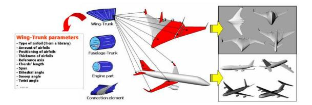
**Figure 5.1** – High level primitive modelling approach that allows to generate variants of a model [LA ROCCA AND VAN TOOREN, 2005].
