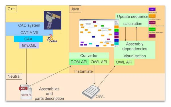
Figure 11.1 – Architecture of the developed software related to the data extraction, dependencies visualisation tool and update sequence computation.
