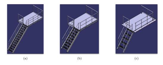
Figure 1.2 – Design variants generated by parameter changes within CATIA V5 CAD system.
