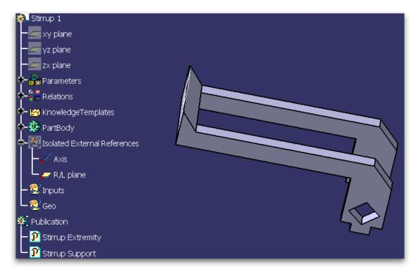
Figure E.1 – Screenshot of a CAD model under CATIA V5.
