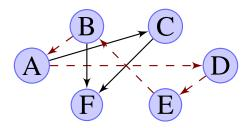
Figure 4.3 – Cycle in a graph. The dashed red arrows from a cycle.
