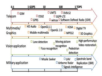
Figure 1.1: Different embedded applications performance requirements grouped by application domain (GOPS: Giga Operations Per Second; TOPS: Tera Operations Per Second) [56].
