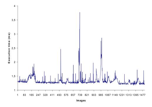
Figure 1.2: Execution time of the connected component labeling algorithm on a video sequence with an Intel Pentium 4 Xeon processor (2.99 GHz) [151].
