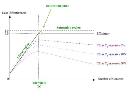
Figure 2.6: Cost-effectiveness of a multithreaded processor when varying  $C_t$  [4].
