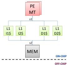
(b) Blocked multithreaded PE with 2 TCs and with 1-level segmented cache memory and on-chip main memory. The L1 I\$ and D\$ memories are segmented per TC
