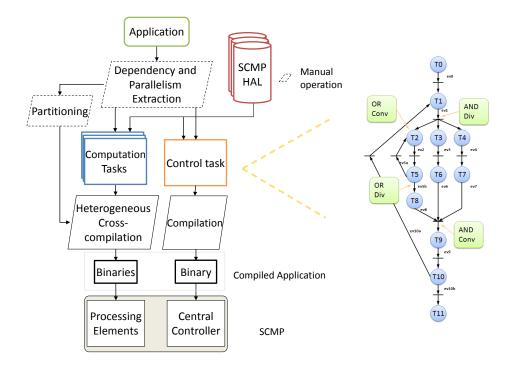
Figure 1.7: SCMP programming model and an example of a typical CDFG control graph.
