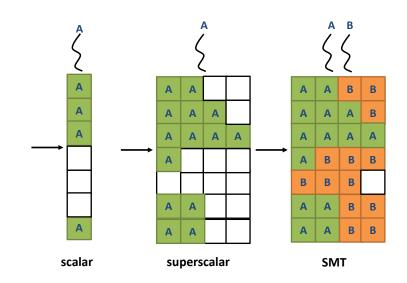
Figure 2.3: Multithreaded processor execution core: scalar, superscalar, SMT. A scalar execution core processes one thread and issues 1 instruction per cycle. On the other hand, a superscalar execution core processes one thread but issues n instructions per cycle depending on the number of functional units. The SMT is a superscalar execution core that processes m threads.
