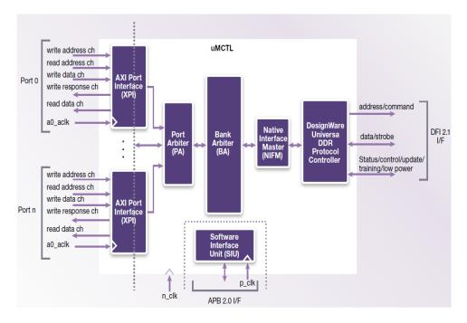
Figure 4.13: DesignWare Universal DDR Memory Controller Block Diagram (Synopsys courtesy).
