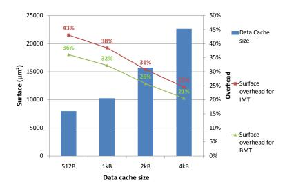
Figure 2.13: MT processor area overhead with respect to the monothreaded processor. Each MT system has one L1 I\$ and one D\$ memory. We show 4 MT systems with different L1 cache sizes. The L1 cache areas are estimated using CACTI 6.5 tool in 40 nm technology and the processors are synthesized in 40 nm TSMC technology.
