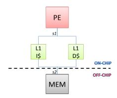
(b) Monothreaded PE with 1-level cache memory and off-chip main memory
