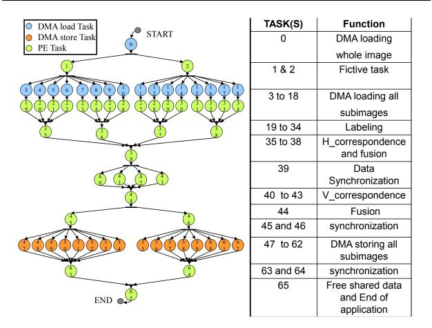
Figure 3.14: CDFG of the connected component labeling algorithm used as input for the centralized control core. The labeling algorithm is decomposed into 16 parallel tasks, where each task performs the labeling algorithm independently on a sub-image.
