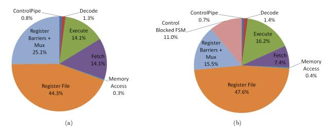
Figure 2.12: Surface repartition of different components synthesized in 40 nm TSMC technology for a) IMT AntX: Total area = 19772  $\mu$ m<sup>2</sup>, Total number of gates = 13.95 kilogates b) BMT AntX: Total area = 18418  $\mu$ m<sup>2</sup>, Total number of gates = 12.99 kilogates.
