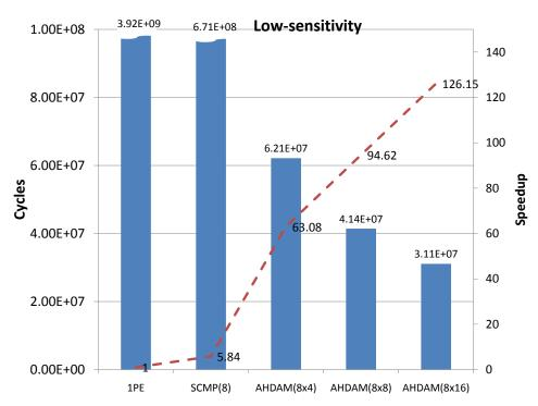
Figure 5.9: Performance of AHDAM v/s SCMP v/s mono for radio-sensing with low-sensitivity. AHDAM architecture has 8 Tiles and 4/8/16 LPEs per Tile. The SCMP architecture has 8 PEs. The real-time deadline of the application is 6 seconds, which corresponds to  $3.10^9$  cycles for 500 MHz processor frequency (much higher than the y-axis scale.
