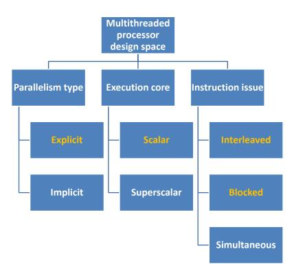
Figure 2.2: Multithreaded processor design space.
