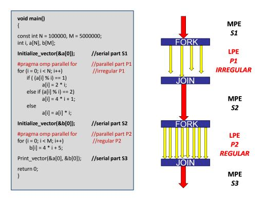
Figure 4.9: A task code example of serial and parallel regions using OpenMP pragmas (fork-join model) allocated by the CCP on a MPE.
