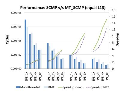
Figure 3.24: Performance and speedup comparison between SCMP v/s MT\_SCMP for control-flow (labeling) application. The number of processors is varied from 1 to 8 and the cache sizes from 1-KB to 8-KB. The cache sizes is per PE.
