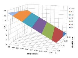
(b) Monothreaded PE CPI with 1-level cache memory and off-chip main memory (50 cy-cles)
