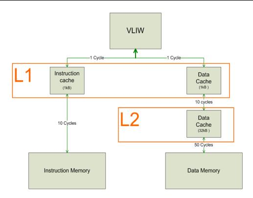
Figure 5.5: Trimaran configuration for modeling the LPE with AHDAM memory hierarchy.
