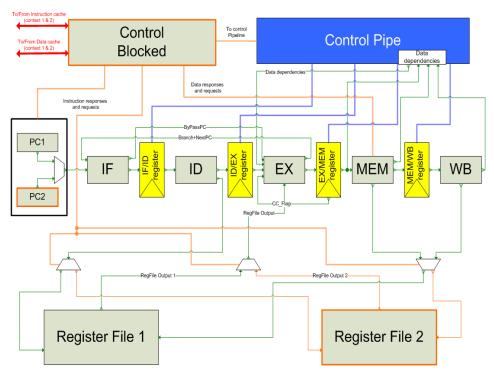
Figure 2.10: Blocked multithreaded AntX.
