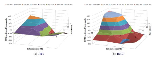
Figure 2.17: Transistor efficiency gain of MT AntX processor with respect to monothreaded AntX processor. For the x-axis, we vary the L1 D\$ size and for the y-axis we vary the data memory latency in cycles.
