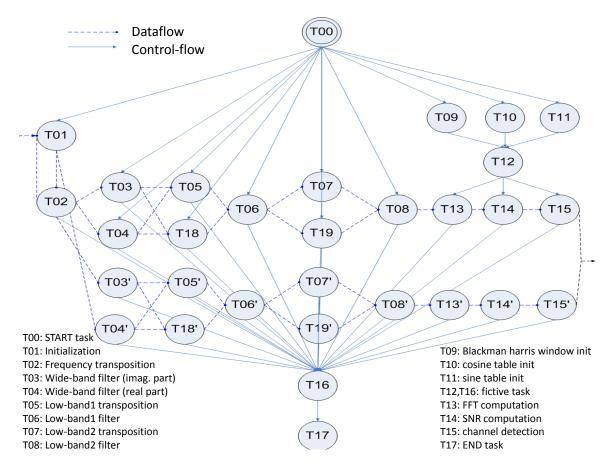
Figure 5.3: CDFG of the radio-sensing application.
