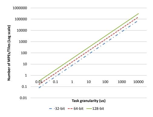
Figure 4.11: Total number of MPEs supported by a 32/64/128-bit control bus. The task granularity (x-axis) varies from 0.01 to 100  $\mu$ s. The y-axis (log scale) shows the total number of MPEs that can be supported by the control bus.
