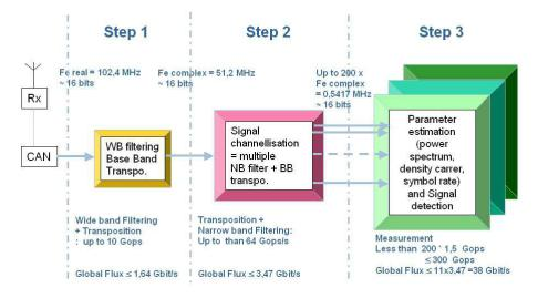
Figure 5.2: Spectrum Sensing main steps, maximal flows and complexities.
