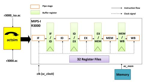
Figure 3.7: R3000 cycle-accurate model generation by actsim tool.
