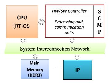
Figure 1.4: SCMP system architecture: the host CPU dispatches massively parallel dynamic applications to SCMP for optimal transistor/energy efficient acceleration.
