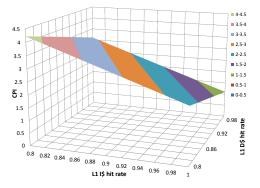
(d) Monothreaded PE CPI with 1-level instruction cache memory and on-chip instruction main memory (10 cycles) and 2-levels data cache memory (10 cycles) and off-chip data main memory (50 cycles)
