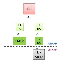
(d) Monothreaded PE with 1-level instruction cache memory and on-chip instruction main memory and 2-levels data cache memory and off-chip data main memory
