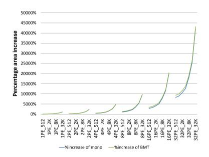
Figure 3.22: Percentage area increase of SCMP with number of processors varying from 1 to 32 and L1 cache size varying from 1-KB to 32-KB. The processors can be monothreaded and BMT. The percentage area increase is compared with respect to the initial SCMP system: 1 monothreaded PE and 1-KB L1 cache memories.
