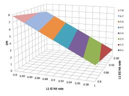
(c) Monothreaded PE CPI with 2-levels cache memory (L2 access=10 cycles) and offchip main memory (50 cycles)
