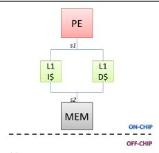
(a) Monothreaded PE with 1-level cache memory and on-chip main memory
