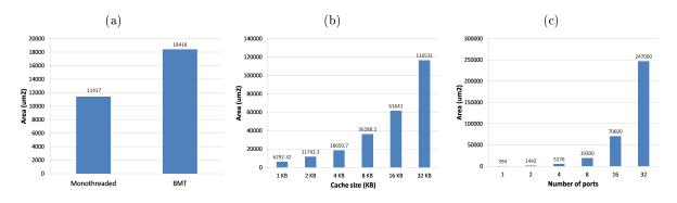
Figure 3.21: Components area in 40 nm technology for a) AntX processor monothreaded and BMT (TSMC) b) L1 cache memory with 16 Byte line and direct-mapped (CACTI 6.5) c) Multibus interconnection network with variable number of I/O ports (TSMC).
