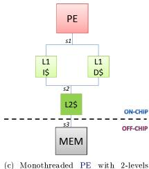
(c) Monothreaded PE with 2-levels cache memory and off-chip main memory
