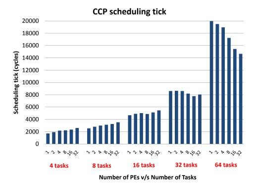
Figure 4.12: CCP scheduling tick length for variable number of PEs (1-32) and tasks (4-64). The application is the connection component labeling with variable levels of parallelism (4-64).
