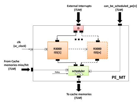
Figure 3.10: Multithreaded ISS model [16].
