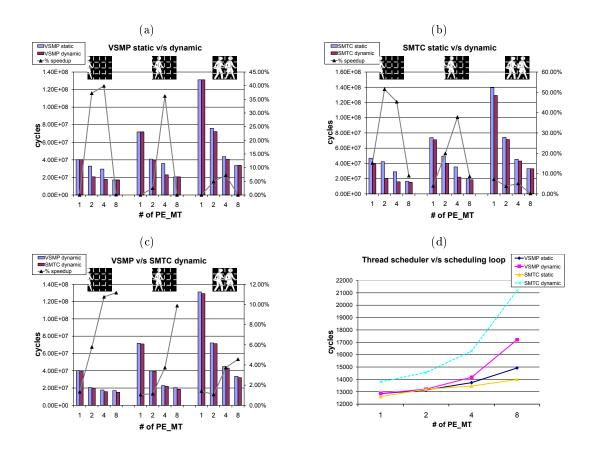
Figure 3.20: Performance comparison of the different thread scheduling strategies: a) VSMP static v/s dynamic. b) SMTC static v/s dynamic. c) VSMP dynamic v/s SMTC dynamic. d) Thread scheduler v/s number of clock cycles per scheduling tick. The speedup line in the first 3 figures is the speedup with respect to the same configuration.
