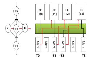
Figure 1.9: Streaming execution model. Each arrow represents an interconnection through the data network between a Processing Element (PE) and a data stored in local memories (Mem). Dark arrows are read/write accesses, whereas gray arrows represent read-only accesses. Task execution begins as soon as intermediate data are ready. Local synchronization is afforded through a memory management unit.
