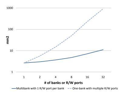
Figure 4.4: Estimated surface of multi-banked memories with 1 R/W port v/s one-bank memory with multiple R/W ports for a 1-MB memory. We vary the number of banks and R/W ports from 1 to 32. The tool used is CACTI 6.5 in 40 nm technology. The surface in  $mm^2$  is plotted as log-scale.
