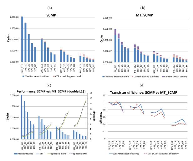
Figure 3.23: Performance of SCMP v/s MT\_SCMP for control-flow (labeling) application. The number of processors is varied from 1 to 8 and the cache sizes from 512-B to 8-KB. The cache sizes is per TC. 1PE\_1K means The performance is plotted in clock cycles a) SCMP system performance b) MT\_SCMP system performance c) Comparison between SCMP and MT\_SCMP performance and speedups d) Transistor efficiency of SCMP and MT\_SCMP with respect to initial system: 1 PE and 512 Byte cache size.
