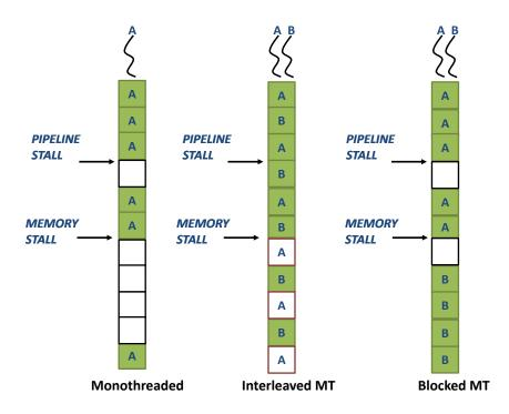
Figure 2.4: Multithreaded instruction issue types compared with monothreaded: interleaved multithreading (IMT), blocked multithreading (BMT). IMT issues an instruction from a different thread at every clock cycle with zero context-switching overhead. On the other hand, BMT allows a thread to run normally as in sequential mode before being switched out for long latency events. However, the context-switching has some penalty cycles.
