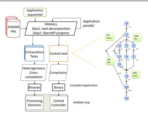
Figure 4.2: AHDAM programming model and an example of a typical CDFG control graph.
