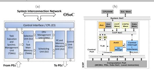
Figure 1.6: a) HW RTOS OSoC [150] b) Programmable RTOS CCP.
