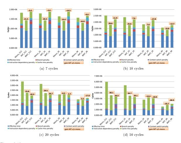
Figure 2.16: Performance results in cycles of monothreaded v/s IMT/BMT AntX with a variable L2 data memory latency. The L1 D\$ size varies from 512-B to 4-KB. L1 cache memories are segmented per TC for the IMT/BMT.
