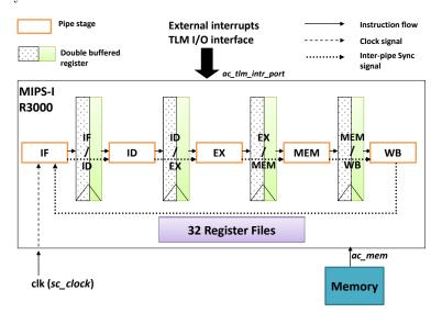
Figure 3.9: New R3000 cycle-accurate model for SoC simulator integration capabilities [15].
