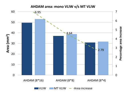
Figure 5.13: AHDAM architecture surface with monothreaded VLIW and multithreaded VLIW for 8 Tiles and 4/8/16 LPEs per Tile.
