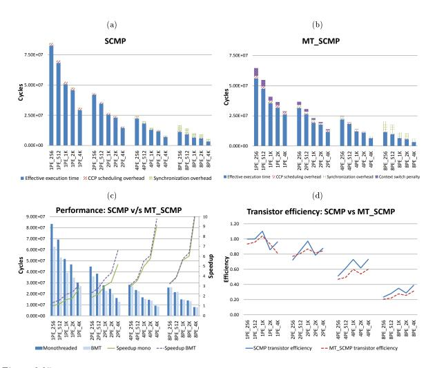
Figure 3.25: Performance of SCMP v/s MT\_SCMP for streaming (WCDMA) application. The number of processors is varied from 1 to 8 and the cache sizes from 256-B to 4-KB. The performance is plotted in clock cycles a) SCMP system performance b) MT\_SCMP system performance c) Comparison between SCMP and MT\_SCMP performance and speedups d) Transistor efficiency of SCMP and MT\_SCMP with respect to initial system: 1 PE and 256-B cache size.
