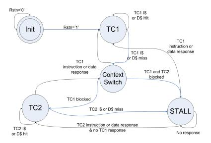
Figure 2.11: Blocked multithreaded AntX FSM for 2 thread contexts: TC1 and TC2. The FSM shows that the BMT processor has 4 execution states: executing TC1, executing TC2, context switching, and stall.
