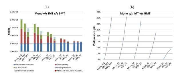
Figure 3.19: Performance results of MT\_SCMP with 1 processor: Monothreaded v/s IMT v/s BMT. The sizes of the L1 I\$ and D\$ are varied simultaneously between 512-B and 8-KB. The performance gain of each multithreaded processor with respect to the monothreaded is plotted in b).
