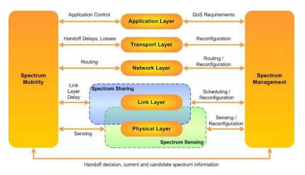
Figure 5.1: Spectrum Sensing description (source EDA/CORSAMA consulting).
