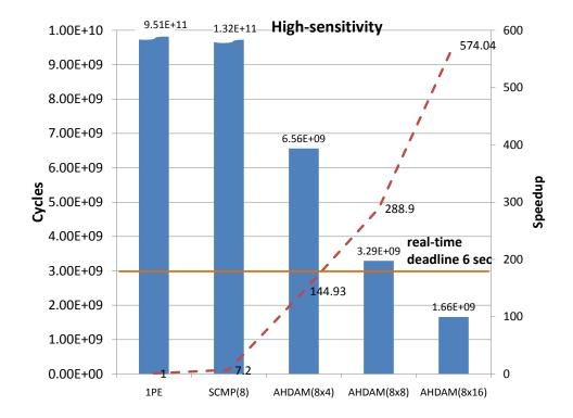
Figure 5.10: Performance of AHDAM v/s SCMP v/s mono for radio-sensing with high-sensitivity. AHDAM architecture has 8 Tiles and 4/8/16 LPEs per Tile. The SCMP architecture has 8 PEs. The real-time deadline of the application is 6 seconds, which corresponds to  $3.10^9$  cycles for 500 MHz processor frequency.
