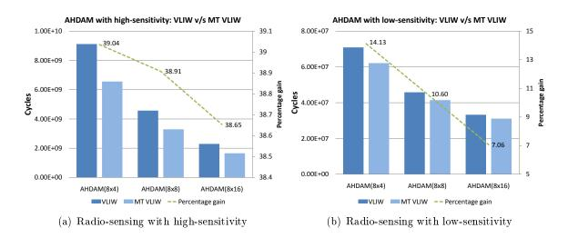
Figure 5.8: Performance of AHDAM architecture with LPE as monothreaded 3-way VLIW v/s multithreaded 3-way VLIW. AHDAM architecture has 8 Tiles and 4/8/16 LPEs per Tile. Performance results and gain are shown for radio-sensing with a) high-sensitivity b) low-sensitivity.
