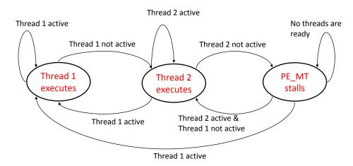
Figure 3.13: Blocked multithreading scheduler FSM using greedy protocol (Moore machine).
