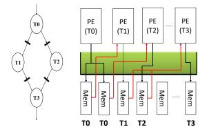
Figure 1.8: Control-flow execution model. Reads and writes are non-blocking. Each arrow represents an interconnection through the data network between a Processing Element (PE) and a data buffer stored in local memories (Mem). Dark arrows are read/write accesses, whereas gray arrows represent read-only accesses. Task execution requires only data produced by tasks that have finished their execution on a PE.
