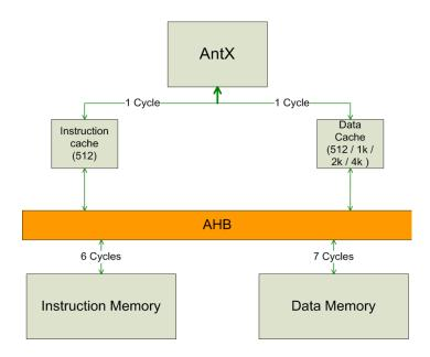
Figure 2.14: AntX hierarchical memory system: Only the data cache size parameter is varied from 512-B to 4-KB. The average memory access latency for the instruction and data memories are observed during application execution and depends on the AHB arbiter. If AntX is multithreaded, then the L1 I\$ and D\$ memories are segmented per TC, which means each TC has half the L1\$ size compared to the monothreaded AntX.
