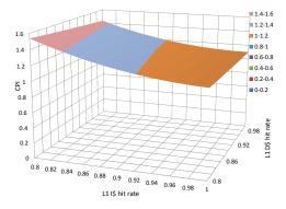
(a) Blocked Multithreaded with 2 TCs' CPI with 1-level instruction cache memory and on-chip instruction main memory and 2-levels data cache memory and off-chip data main memory. The L1 I\$ and D\$ are segmented per TC
