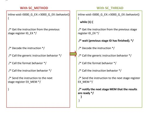
Figure 3.8: Pseudo-code for the EX-stage module in ArchC 2.0.
