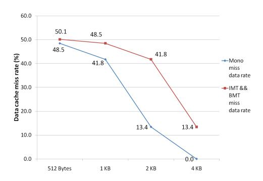
Figure 2.15: Data cache miss rates for monothreaded and IMT/BMT AntX while varying the cache size: 512-B, 1-KB, 2-KB, and 4-KB.
