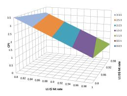
(a) Monothreaded PE CPI with 1-level cache memory and on-chip main memory (10 cy-cles)
