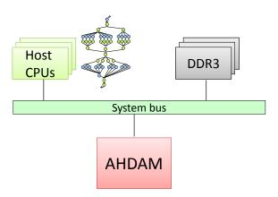
Figure 4.1: AHDAM system environment: multiple host CPUs offloading massively-parallel applications to the AHDAM architecture. The large data set is stored in multiple off-chip DDR3 memories.
