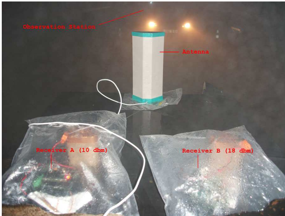
Figure 3.40: The receiver LiveNodes at the night room during experiment
