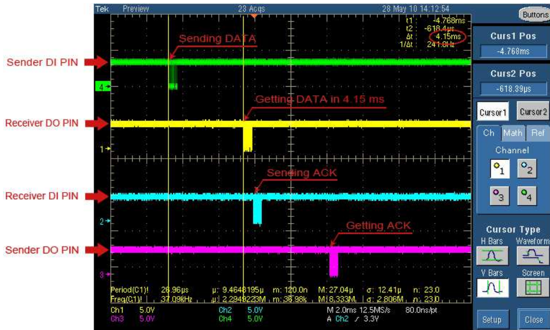
Figure 3.32: Delays when sending and receiving a message in five octets
