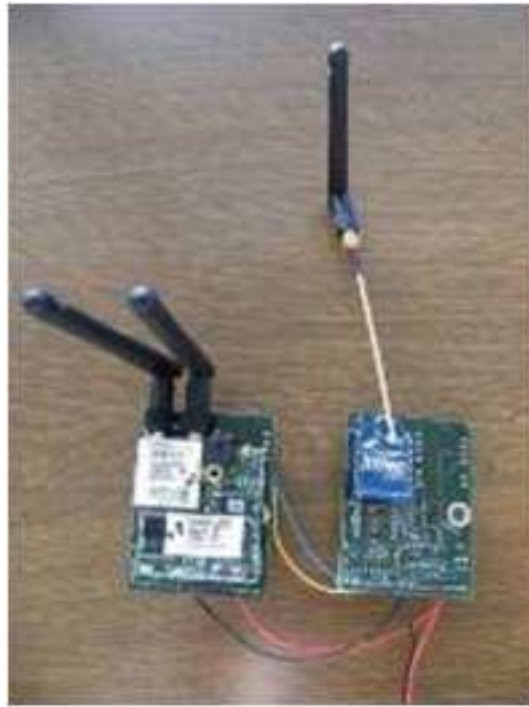
Figure 3.21: Two LiveNode sensors link together: ZigBee plus Wi-Fi
