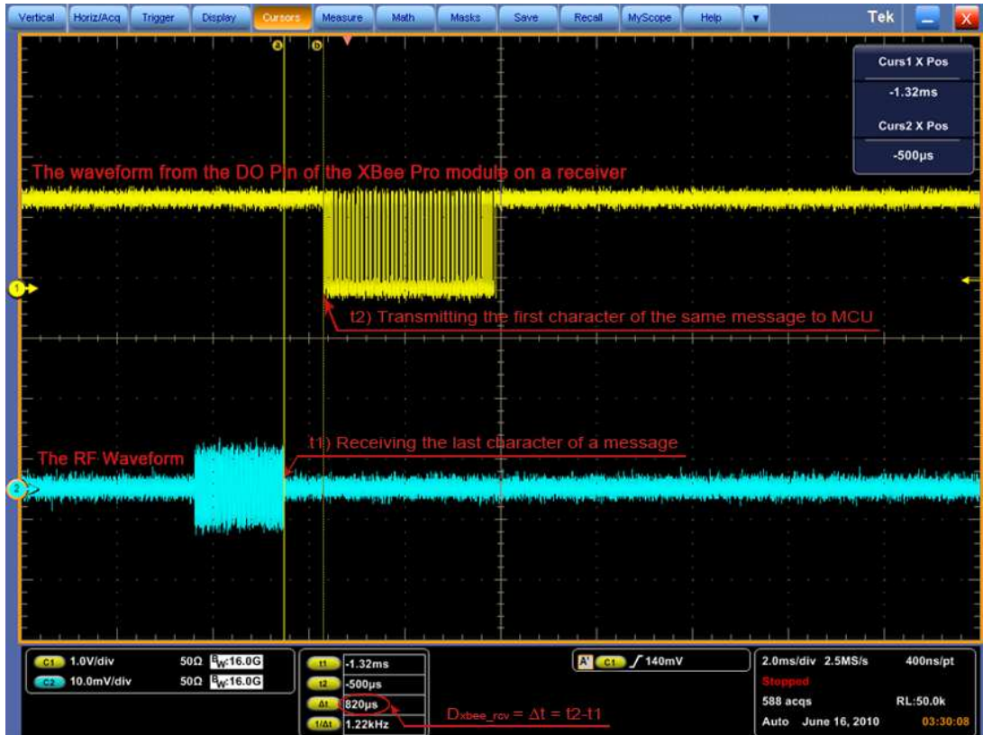
Figure 3.30: The waveforms in the receiving process
