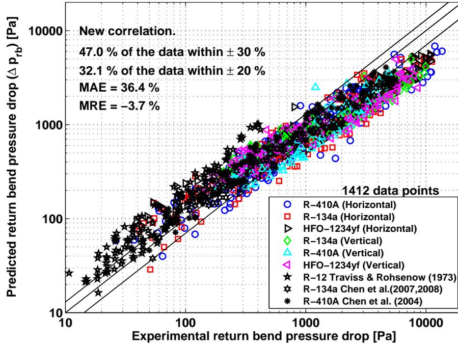
Figure 6.19: Comparison of 1412 data points with predictions by the proposed correlation.
