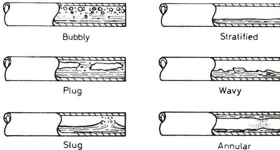
Figure 3.2: Two-phase flow patterns in horizontal flow [Collier & Thome 1994].
