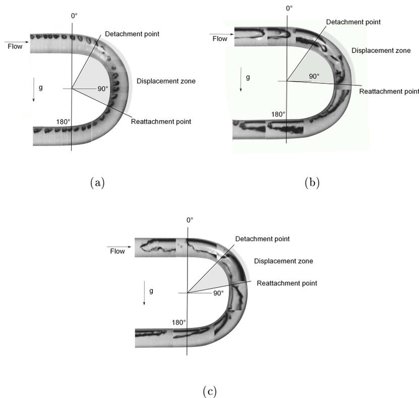
Figure 6.8: Visual reconstitution of bubble, slug head and slug tail behaviors and trajectories during a vertical downward flow in a return bend. Test conditions are  $x = 5\%$ ,  $G = 300 \text{ kg}\cdot\text{m}^{-2}\cdot\text{s}^{-1}$ ,  $T_{\text{sat}} = 10 \text{ }^\circ\text{C}$  and  $D = 6.70 \text{ mm}$ .
