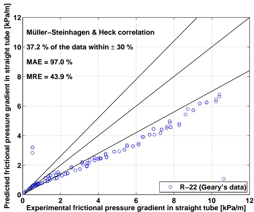
Figure 3.8: Comparison made by [Padilla *et al.* 2009] between the experimental frictional pressure gradient in straight tubes from [Geary 1975] and the predicted one by [Müller-Steinhagen & Heck 1986].
