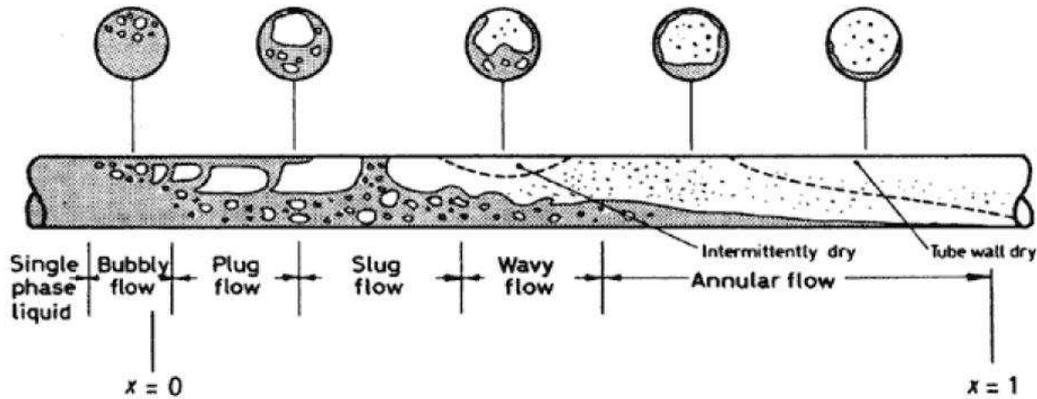
Figure 3.4: Flow patterns during evaporation in a horizontal tube [Thome 2004].
