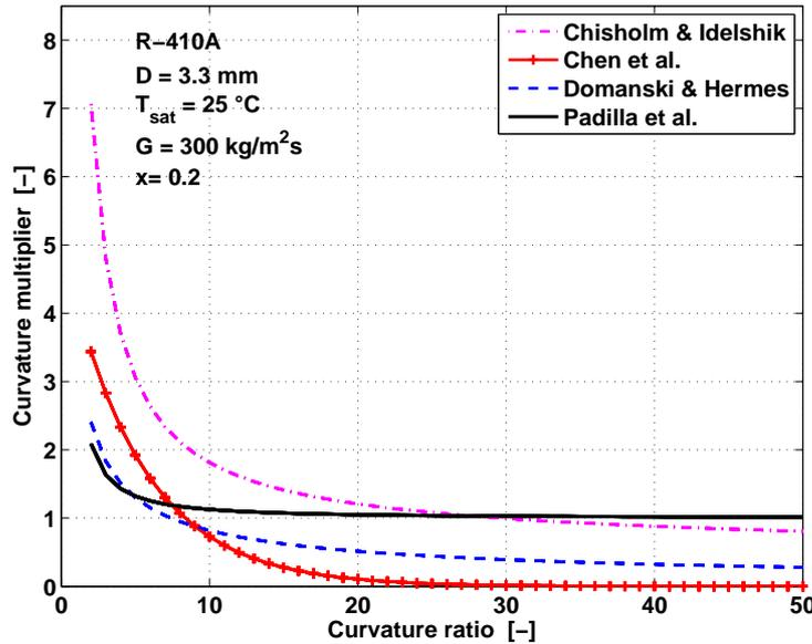
Figure 3.10: Curvature multiplier  $\left(\frac{dp}{dz}\right)_{rb} / \left(\frac{dp}{dz}\right)_{st}$  as a function of the curvature ratio ( $2R/D$ ) for the [Padilla *et al.* 2009] prediction method and different correlations from the literature. [Padilla *et al.* 2009]
