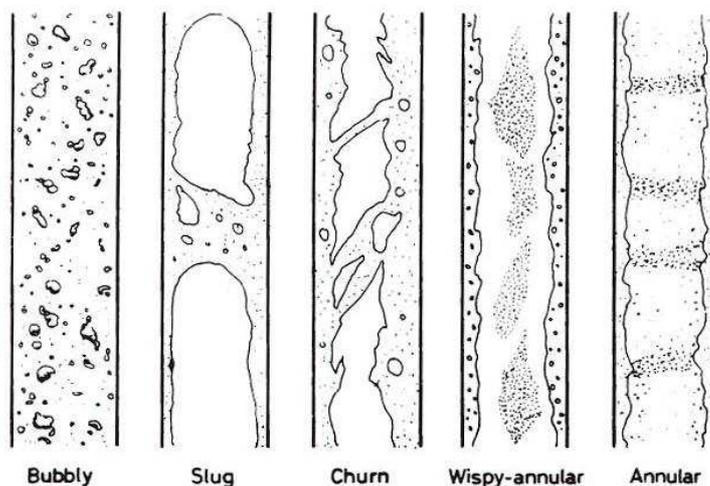
Figure 3.3: Two-phase flow patterns in vertical flow [Collier & Thome 1994].
