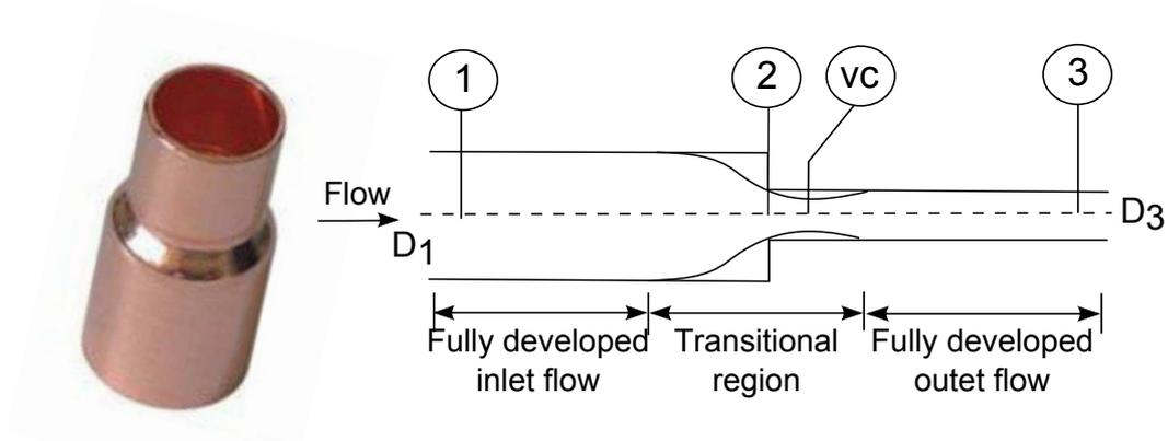
Figure 2.4: Single-phase flow through a sudden contraction.
