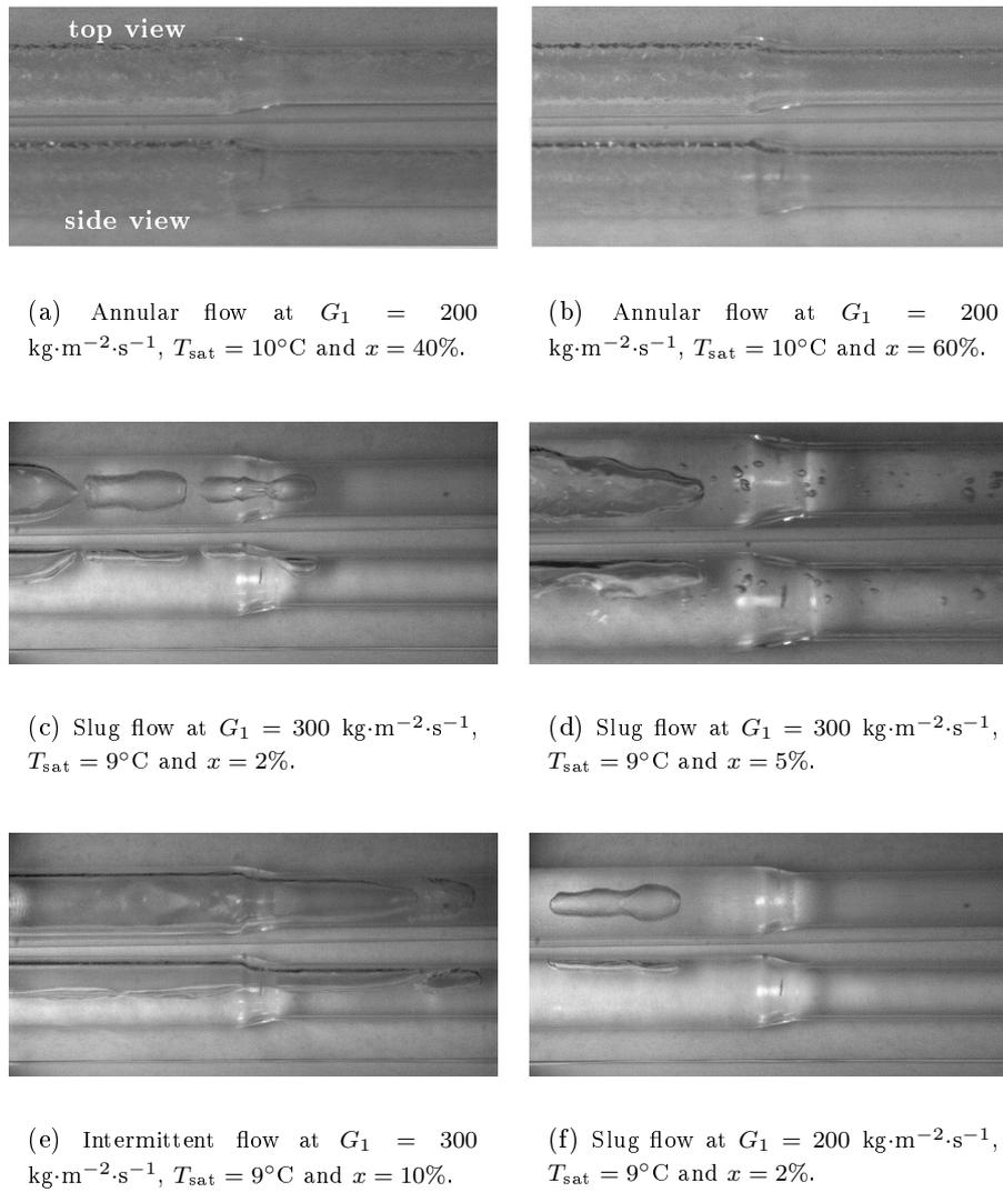
Figure 7.2: Side and top views of the R-134a flow patterns in a horizontal sudden contraction.  $D_1 = 10 \text{ mm}$ ,  $\sigma_A = \frac{D_2^2}{D_1^2} = 0.49$ .
