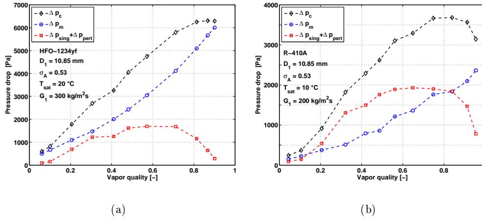
Figure 7.7: Pressure drop contributions vs. vapor quality.
