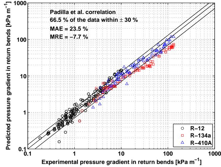
Figure 3.9: Experimental pressure gradient data for return bends (Table 3.1) compared to the [Padilla *et al.* 2009] prediction method.
