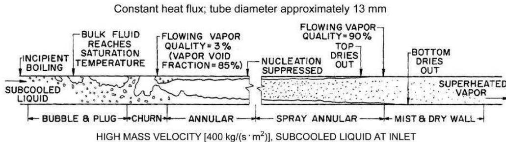
Figure 3.1: Flow regimes in typical evaporator smooth horizontal tube [ASHRAE 2001].
