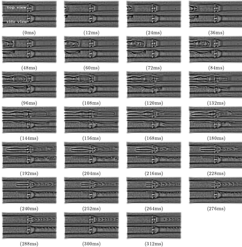
Figure 7.3: Side and top views progress of R-134a slug flow along a sudden contraction for  $x = 1\%$ ,  $G_1 = 200 \text{ kg}\cdot\text{m}^{-2}\cdot\text{s}^{-1}$ ,  $T_{\text{sat}} = 8 \text{ }^\circ\text{C}$ ,  $D_1 = 10.0 \text{ mm}$  and  $\sigma_A = \frac{D_2^2}{D_1^2} = 0.49$ .
