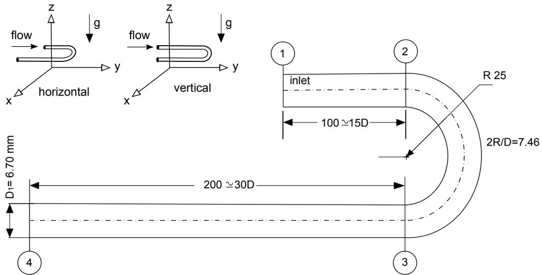
Figure 4.3: Sketch of the test section for flow regime visualizations in return bends.
