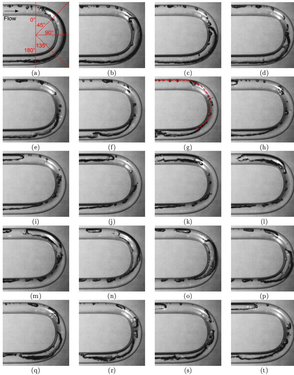
Figure 6.7: Side view progress of HFO-1234yf slug flow entering at the higher tube (flowing downwards) in a vertical return bend for  $x = 5\%$ ,  $G = 300 \text{ kg}\cdot\text{m}^{-2}\cdot\text{s}^{-1}$ ,  $T_{\text{sat}} = 10 \text{ }^\circ\text{C}$  and  $D = 6.70 \text{ mm}$  (time lapse between images = 15 ms, total time lapse = 0.28 s).
