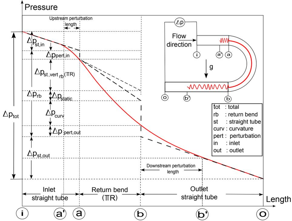
Figure 6.1: Idealized pressure profile along a vertical return bend.
