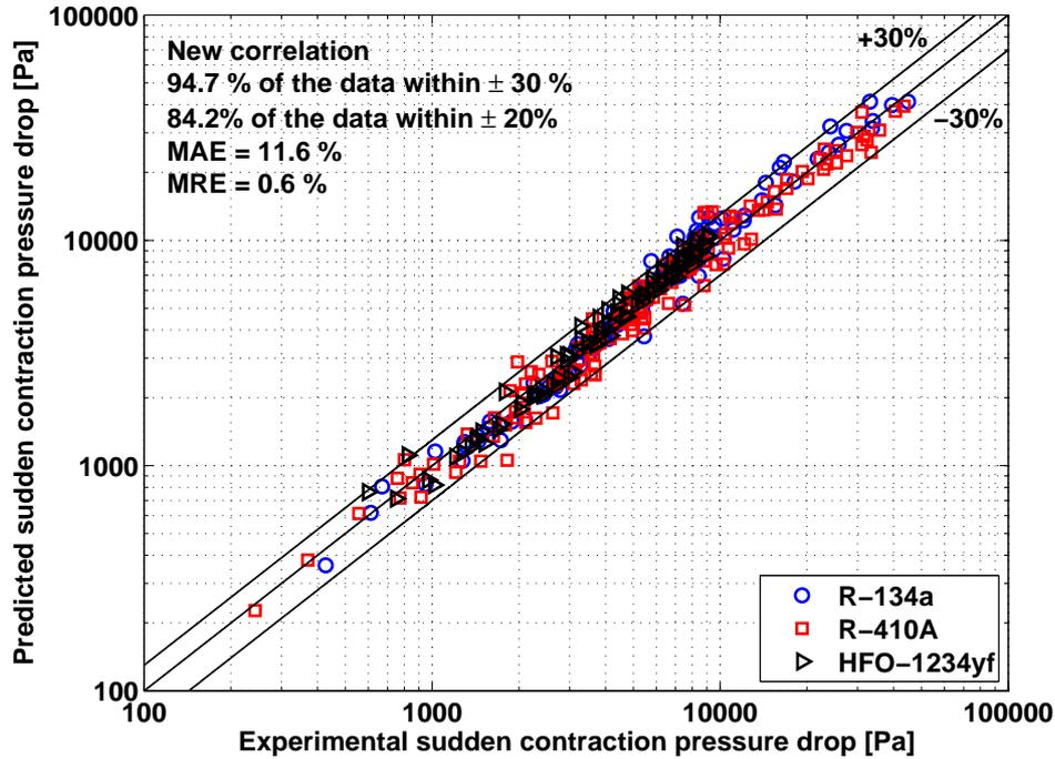
Figure 7.11: Comparison of 360 data points with predictions by the proposed correlation.
