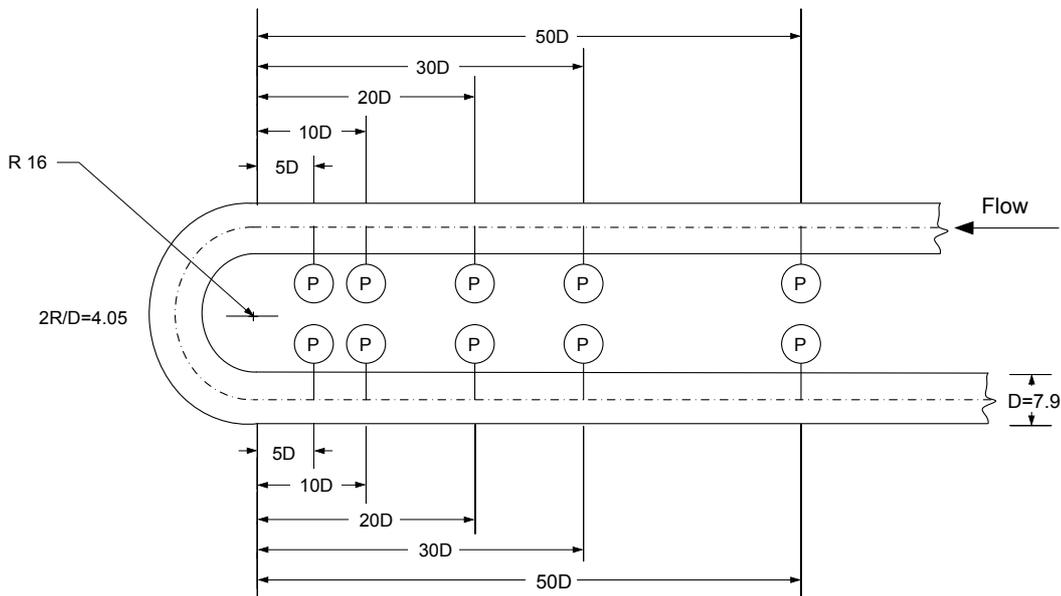
Figure 4.7: Test section used to measure the perturbation lengths up- and downstream of a return bend.
