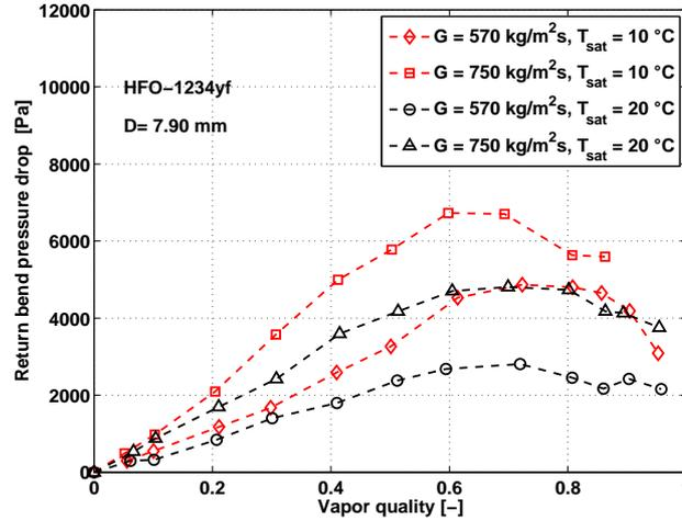
Figure 6.13: Return bend pressure drop vs. vapor quality.
