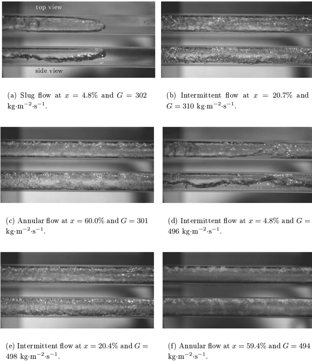
Figure 5.4: Top and side views of the R-134a flow patterns for  $T_{\text{sat}} = 10 \text{ }^\circ\text{C}$  and  $D = 6.70 \text{ mm}$ . [Padilla *et al.* 2011a]
