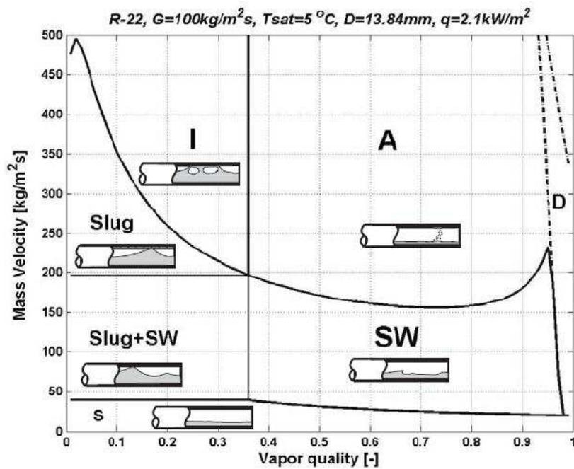
Figure 3.5: Flow pattern map of [Wojtan *et al.* 2005a] for R-22 at  $T_{\text{sat}} = 5^\circ\text{C}$  in a 13.84 mm internal diameter tube at  $G = 100 \text{ kg}\cdot\text{m}^{-2}\cdot\text{s}^{-1}$  and  $q = 2.1 \text{ kW}\cdot\text{m}^{-2}$ . [Quibén 2005]
