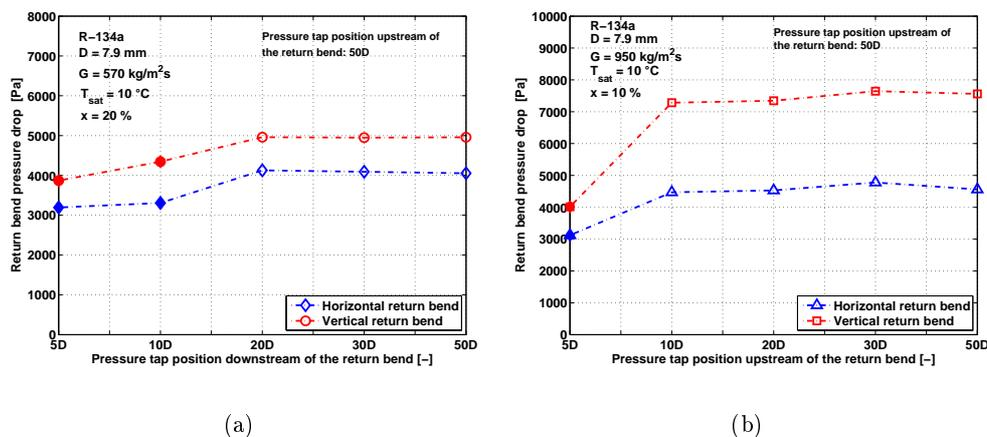
Figure 6.11: Return bend pressure drop as measured at different pressure tap locations ( $5D$ ,  $10D$ ,  $20D$ ,  $30D$  and  $50D$ ) up- and downstream on vertical and horizontal return bends. Filled markers correspond to measurements affected by the perturbation.
