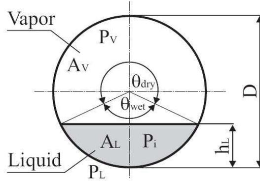
Figure 3.6: Cross-sectional and peripheral fractions in a circular tube. [Quibén 2005]
