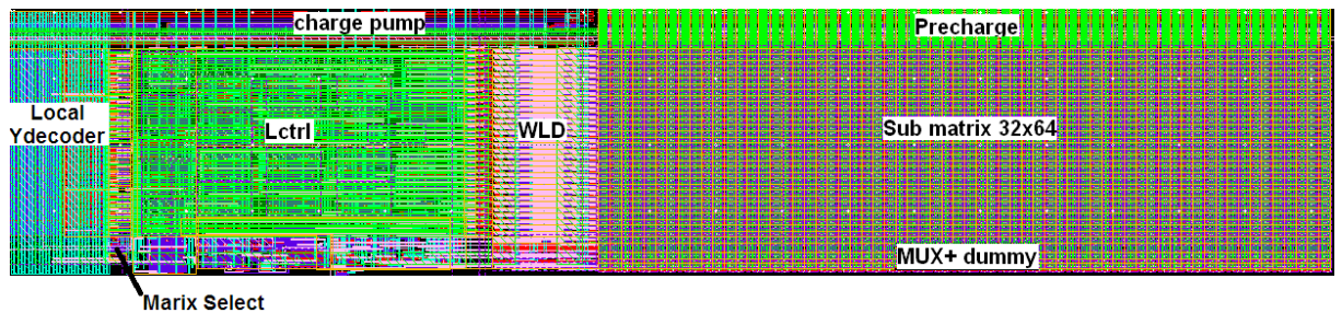
Figure 5.14: Layout of the sub-matrix including Matrix array, Control block, Mux, and Ydecoder
