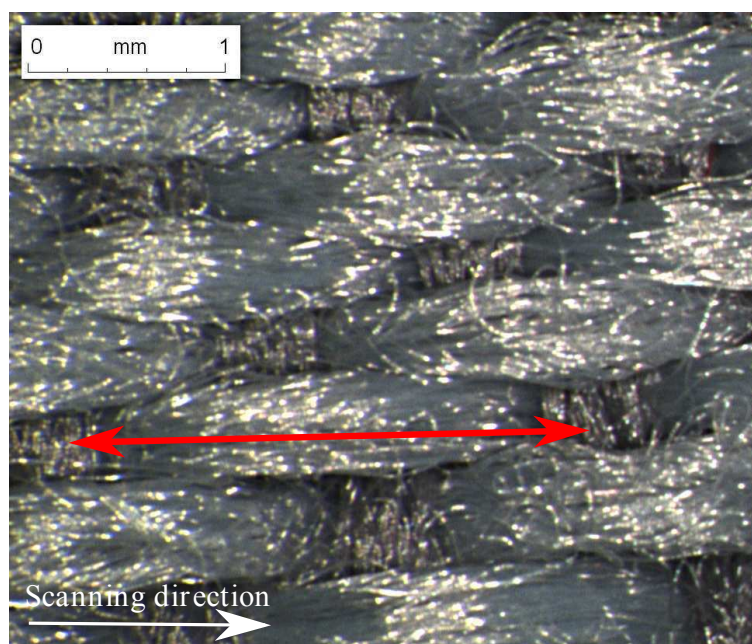
Figure 3.8: Fabric texture. The texture period is 2.2 mm.
