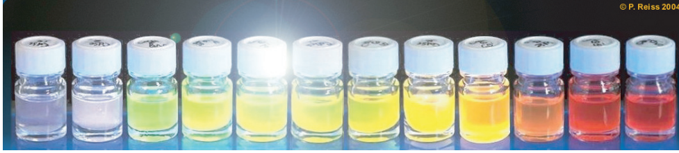
FIGURE I.2 – Emission of CdSe nanocrystals of different sizes While the nanocrystals diameter varies from around 2 nm to 7 nm, the emission of nanocrystals shifts from 480 nm to 650 nm.
