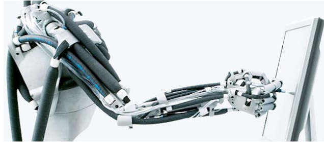
(b) Softech humanoid robot with Festo muscles
