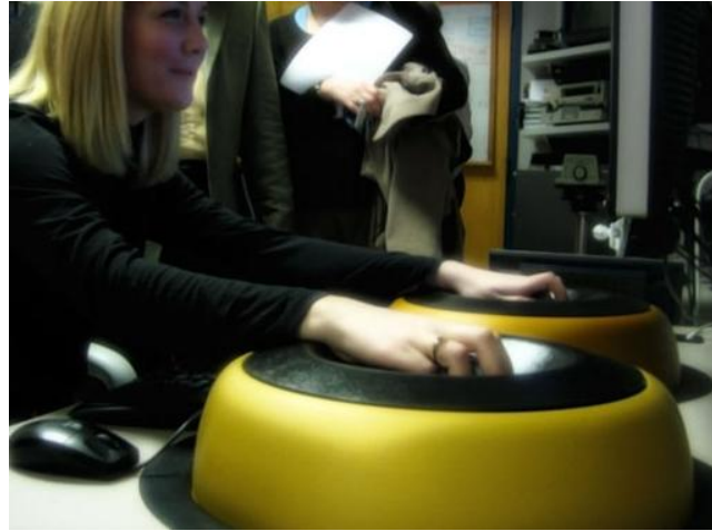
Fig. 1.10. Magnetically levitated device (Carnegie Mellon University)
