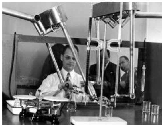
Fig. 2.9. The first teleoperation system developed by (Goertz 1952)
