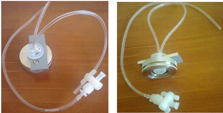
Figure 8.1 Pictures of the two models of flow chamber used for this project. A: a model realised in the laboratory by Philippe Robert, with dimension of 4 \times 4 \times 1 \text{ cm}^3 and the polish bottom to improve the contrast. B: A modified round chamber with teflon insert used for supported lipid bilayer.
