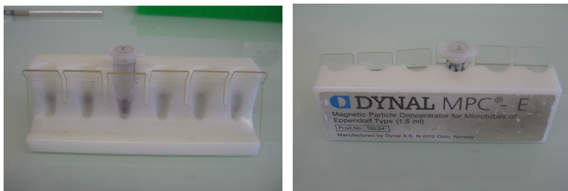
Figure 8.2 Dynal MPC-E magnet. This instrument, which can support six tubes of 1.5 ml, allows to separate the pellet from the supernatant which is repeatedly removed.
