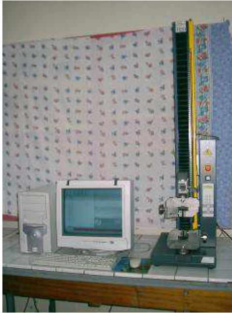
Figure II.7. Machine de traction Zwick
