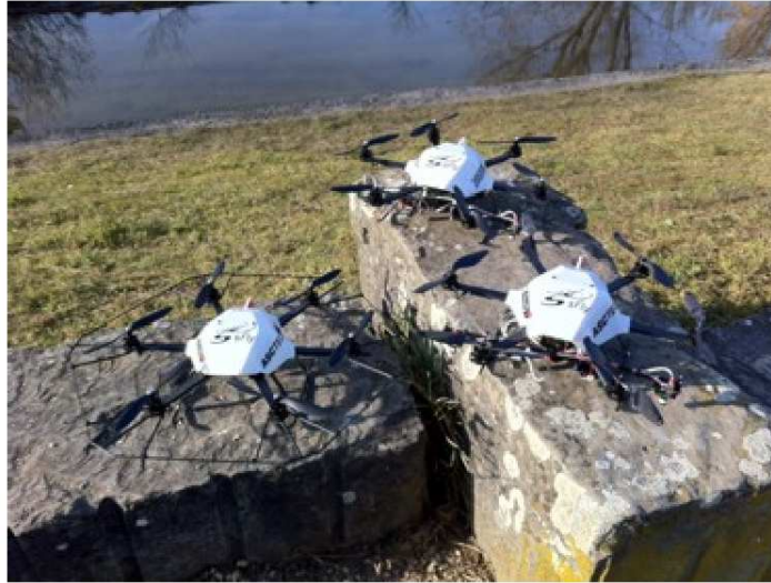
Figure 1.2: ATG delivered the 3 new helicopters version 3 (hexacopters), each one equipped with a Core2Duo computer board, camera mounts, and communication modules (WiseNodes) by the industrial partner CSEM.
