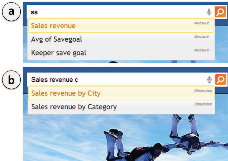
Figure VI.8: Screenshot of auto-completion in the search text box. (a) First suggestions after characters “sa” and (b) suggestions following the selection of measure Sales revenue and character “c”.
