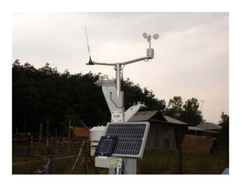
**Figure 12** Local microclimate (Minimet automatic weather station, Skye Instruments Ltd, U.K.) was automatically monitored in an open field, 50 m from any trees.
