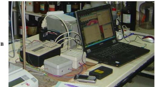
Figure 9 A) Installation of cut stem with a high pressure flow meter (HPFM) and weighing water flowing out of cut segments by 0.01 g accuracy balance.
