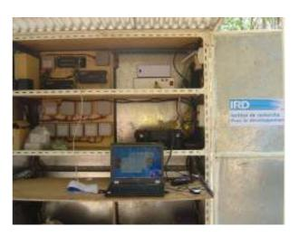
**Figure 10** Installation of xylem sap flow probe in the experimental tree at a height of 1.8 m above the soil and the data logger (CR10X, Campbell Scientific, Leicester, U.K.) with multiplexer setting.
