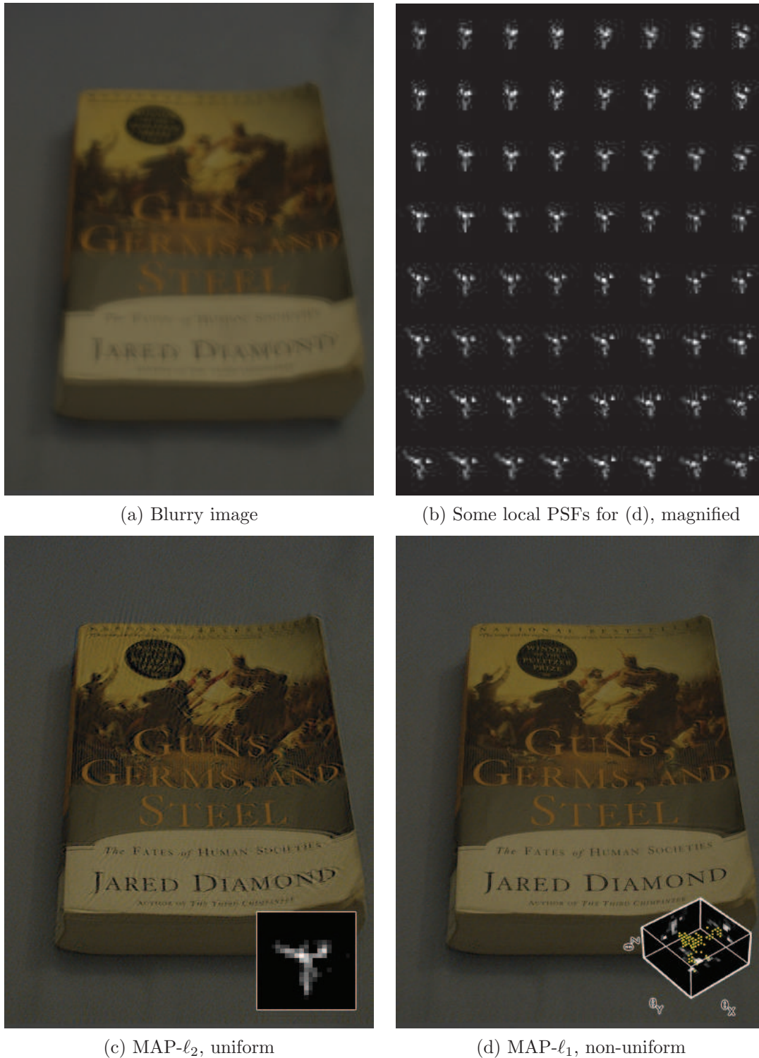
Figure 4.3. Blind deblurring of real camera shake, example 3. The result of blind deblurring on a real camera shake image (a), captured with a shutter speed of 1 second, using the MAP approach of Cho and Lee with both the uniform and non-uniform blur models. Also shown in (b) are some of the local PSFs generated from the blur kernel in (d) at various points in the image. In the blurry image, most of the text on the book cover is too blurred to read. Deblurring the image with the uniform blur model (c) allows some of the text on the cover of the book to be read, however, after deblurring with our non-uniform model (d), all but the smallest text becomes legible. The estimated kernels for the two models are shown inset in the deblurred results. The blur kernel in (d) covers \pm 0.4^\circ in \theta_X and \theta_Y , and \pm 0.9^\circ in \theta_Z .
