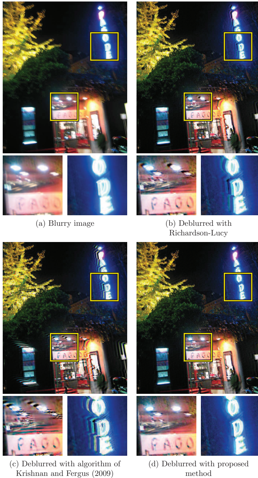
Figure 6.9. Deblurring saturated images. Note that the ringing around saturated regions, visible in columns (b)–(c) is removed by our method (d), without causing any loss in visual quality elsewhere.
