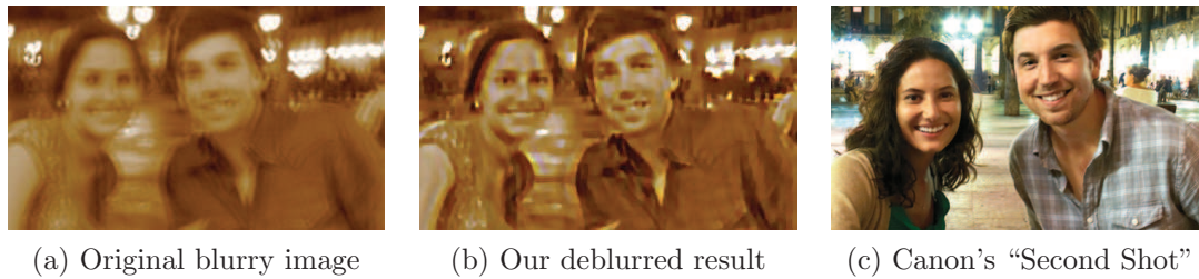
Figure 1.3. Deblurring a real saturated image. Taken from Canon's "Your Second Shot" advertising campaign. The original image (a) is very blurry, however using blind PSF estimation (Chapter 4) to estimate how the image was blurred, followed by non-blind deblurring, handling the saturated pixels (Chapter 6) we are able to obtain a much better image (b). For the advertising campaign, Canon flew the couple back to Barcelona to take the photo again (c) with a new camera.
