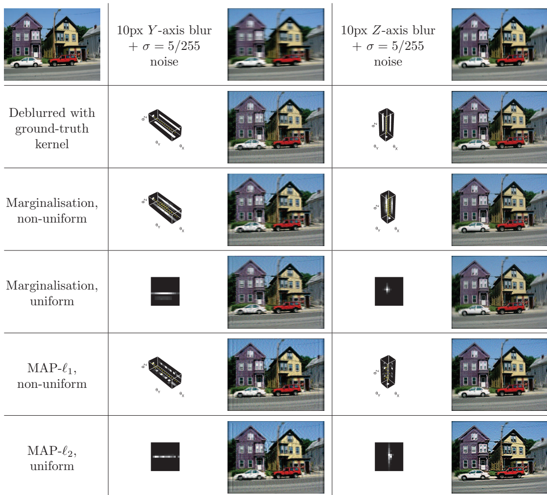
Figure 4.4. Blind deblurring of synthetic single-axis blurs. A sharp image (top left) with examples of synthetic blur by rotation of the camera about its Y and Z-axis, and the kernels and deblurred results for different cases. We compare the results of blind deblurring for two sizes of blur and three noise levels, and the reconstruction errors are summarised in the table at the top. For each single-axis blur, the table contains the root-mean-square (RMS) errors between the deblurred results and the ground-truth sharp image for blurs with a maximum size of 10 or 20 pixels in the image, using our non-uniform model and the uniform model. In each cell we also show, in parentheses, the ratio between the RMS error and the corresponding error for that blurry image deblurred with the ground-truth kernel. Note that to facilitate comparison without the influence of image priors, the deblurred images were all produced using the Richardson-Lucy algorithm.
