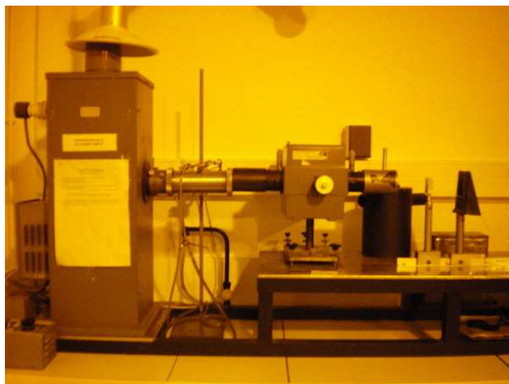
Figure III-C-1 Picture of the monochromatic irradiation device
