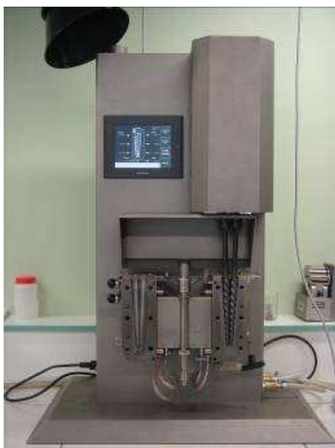
*Figure 3.3. DSM Micro 15 TS Compounder*
