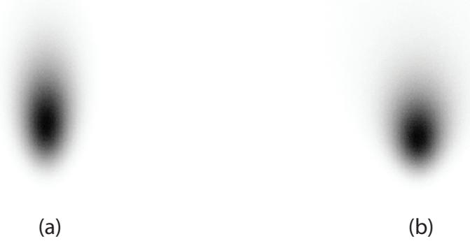
Figure 4.10: A divergent laser beam projects to a plane at an angle of  $28^\circ$
