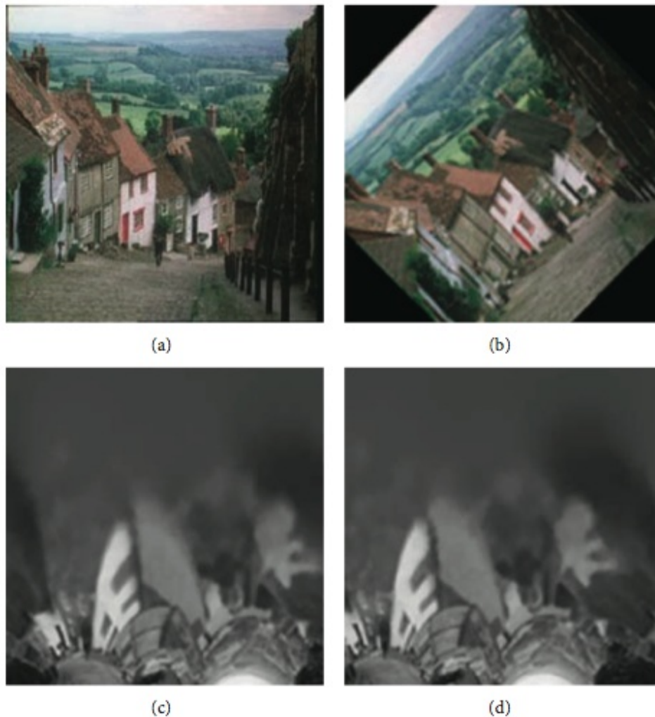
Figure 2.11: Example of how rotation attack affects an image in Cartesian and Log-polar system: a) Original image in Cartesian system; b) Rotated image with 45 degrees in Cartesian system; c) Original image in Log-polar coordinates; d) Rotated image in log-polar coordinates.
