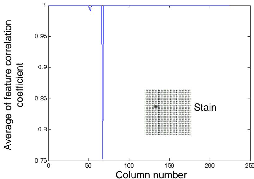
Figure 4.33: Variation of feature correlation due to the presence of a defect
