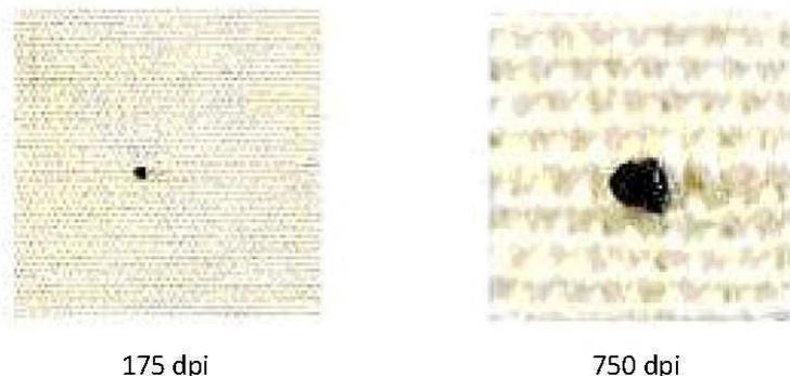
Figure 4.40: Effect of acquisition resolution of fabric image
