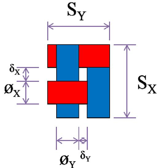
Figure 4.6: Dimensions of fabric basic unit (repeat)
