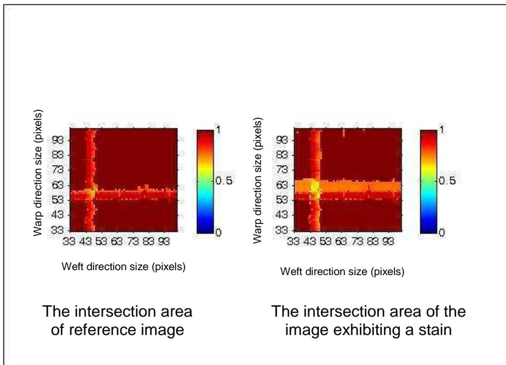
Figure 4.41: Optimization of sub-window size for a simulated image exhibiting a stain
