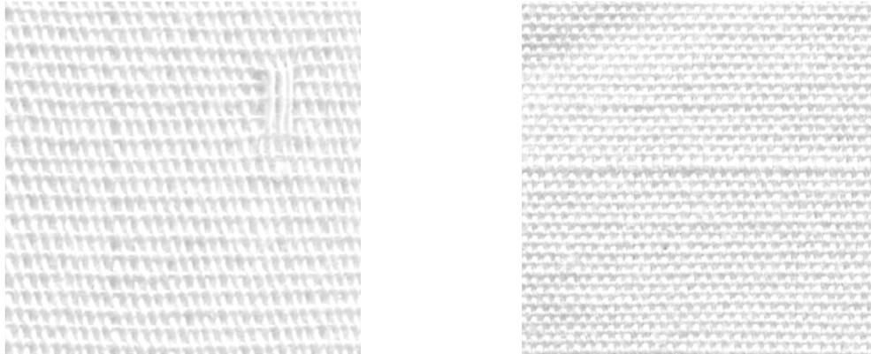
Figure 4.28: Warp-float and coarse-pick
