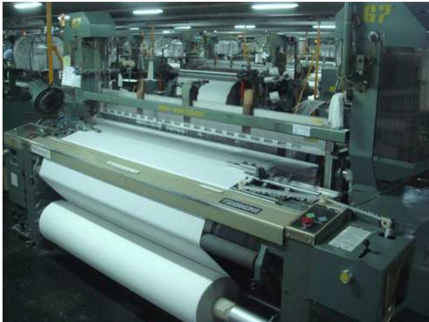
Figure 2.1: Modern (air-jet) looms
