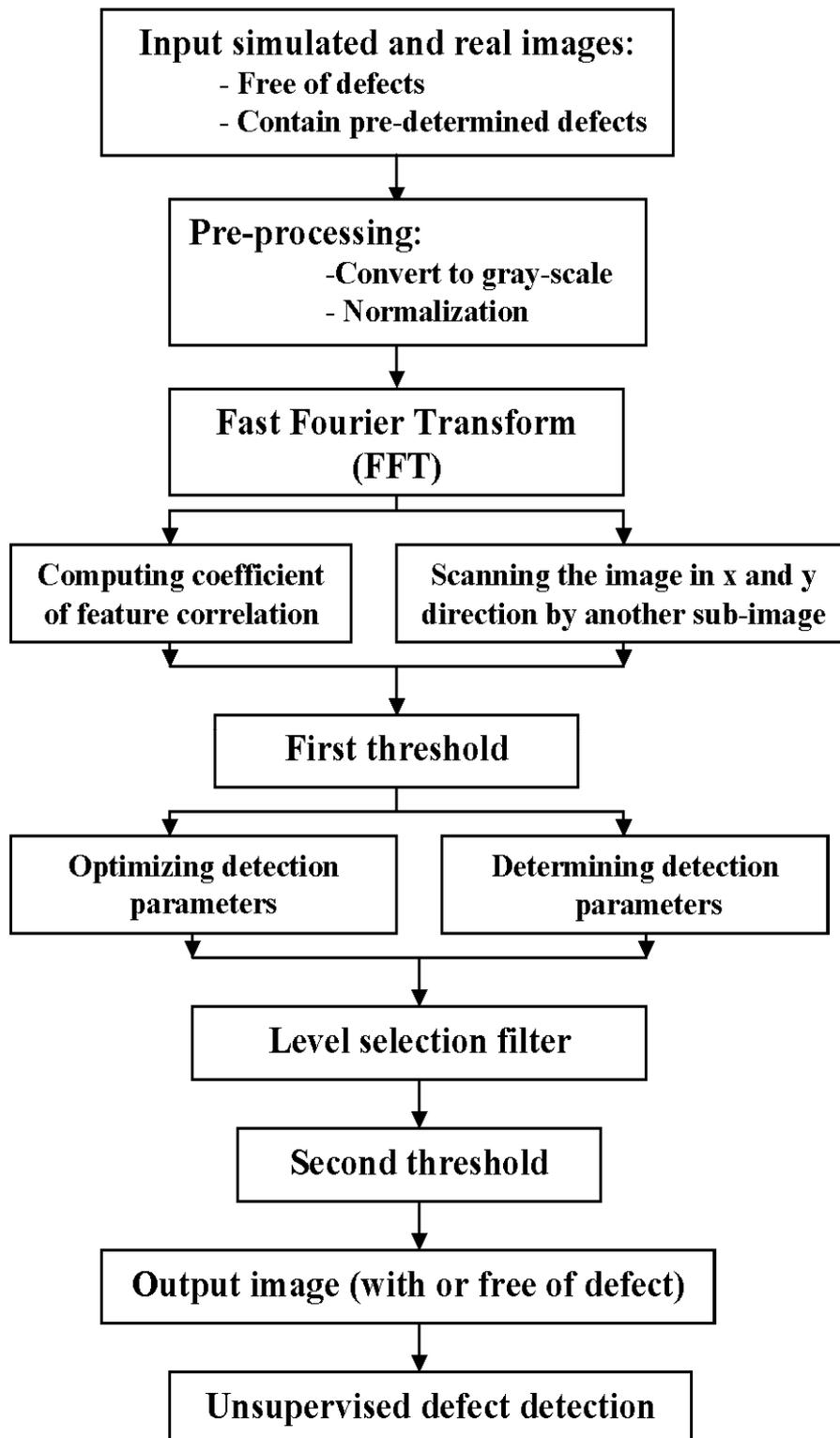
Figure 4.35: Flow-chart of defect detection procedure
