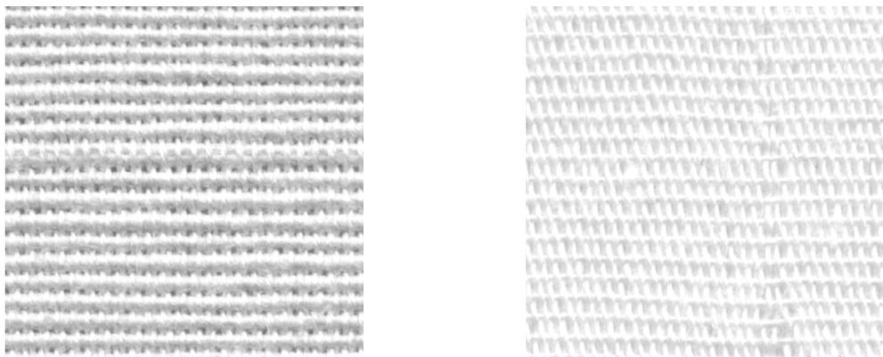
Figure 4.27: Double-pick and double-end
