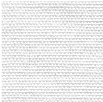
Figure 4.24: Real image of the defect-free plain fabric
