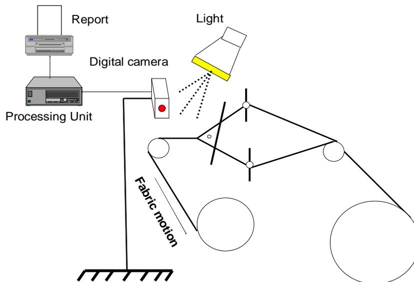
Figure 4.44: The schematic of the vision prototype
