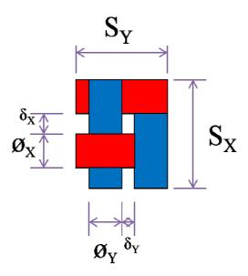
Figure 4.6: Dimensions of fabric basic unit (repeat)
