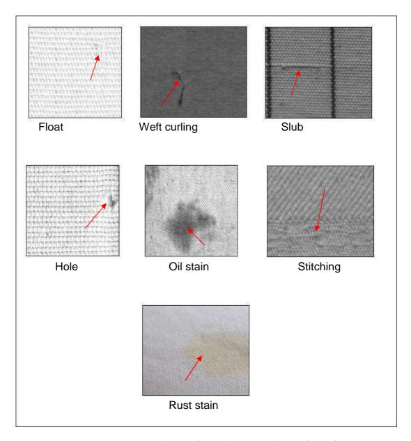
Figure 4.2: The defects of the first part of table (4.1-a)
