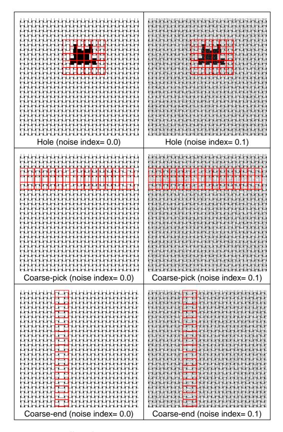
Figure 5.7 Effect of increasing the noise level on detection results
