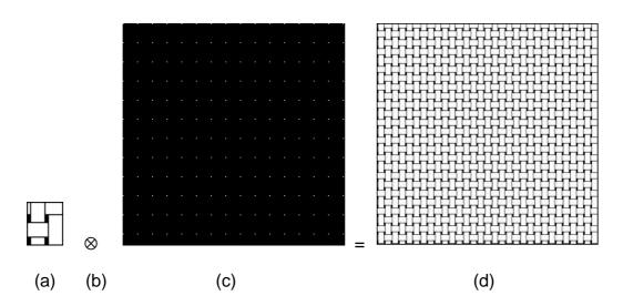
Figure 4.8: (a) basic unit, (b) convolution mask, (c) basic unit repetition, (d) simulated image of the defect-free plain fabric
