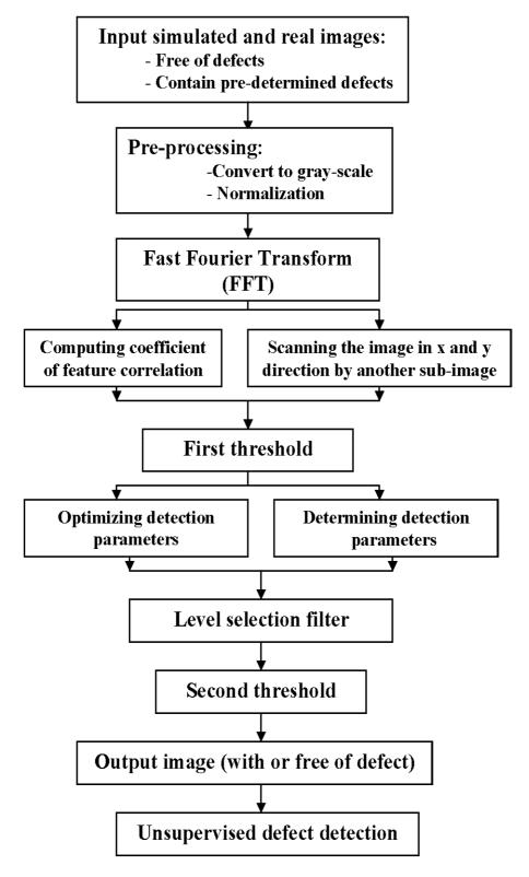
Figure 4.35: Flow-chart of defect detection procedure
