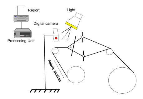
Figure 4.44: The schematic of the vision prototype
