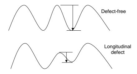
Figure 5.3: Effect of longitudinal defect on Fourier frequency
