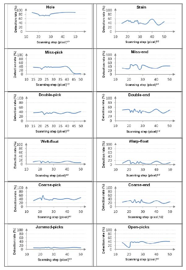
Figure 5.4: Effect of scanning step on defect detection rate for simulated fabric during the optimization
