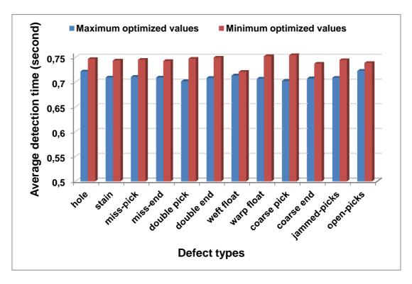
Figure 5.18: The measured detection time for real fabric defect detection
