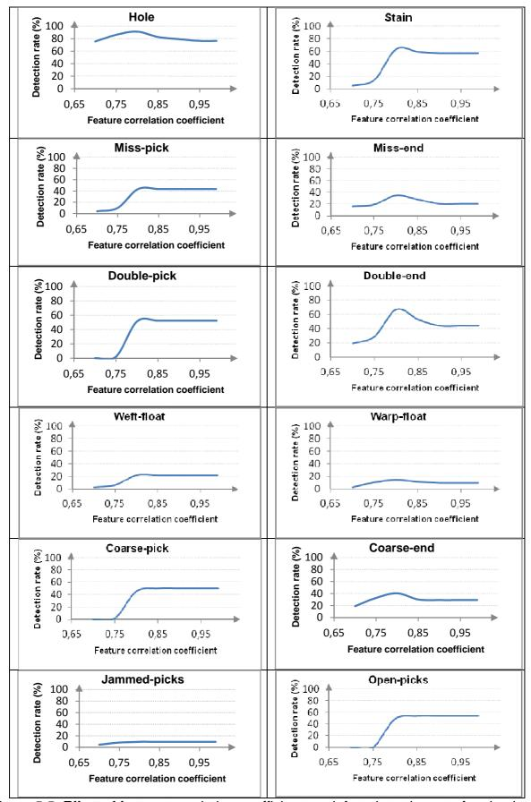
Figure 5.5: Effect of feature correlation coefficient on defect detection rate for simulated fabric
