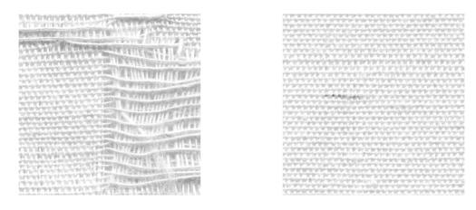
Figure 4.30: Tear and contamination
