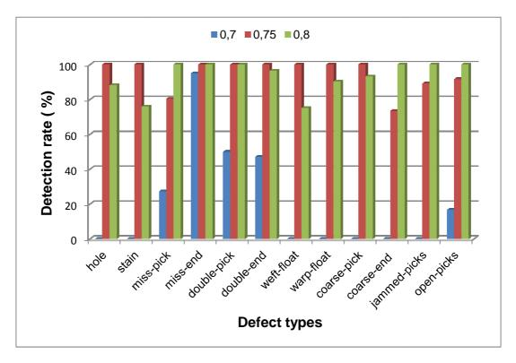
Figure 5.15 Optimization of feature correlation coefficient for real defect detection
