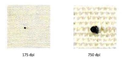
Figure 4.40: Effect of acquisition resolution of fabric image
