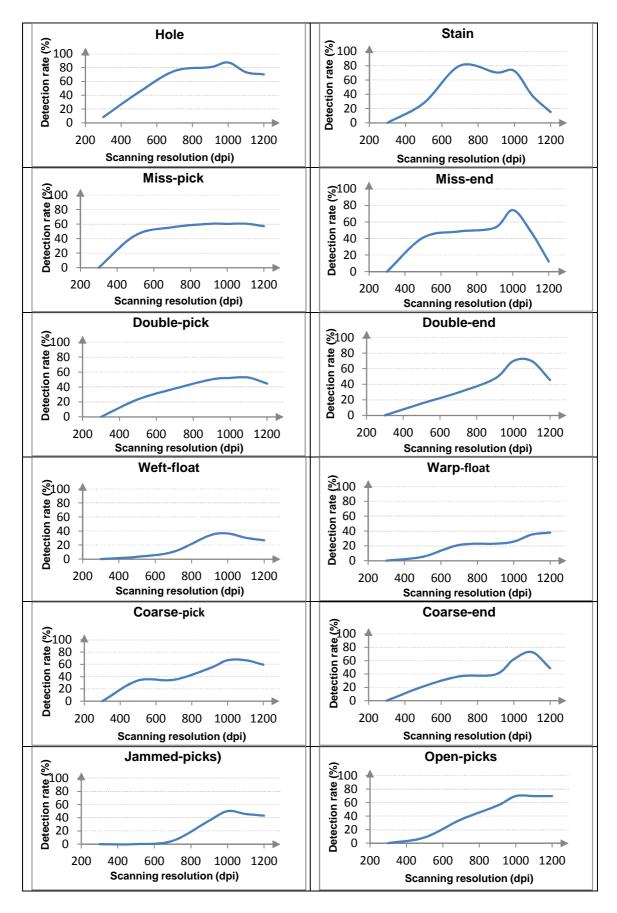
Figure 5.12: Optimization of scanning resolution for real fabric
