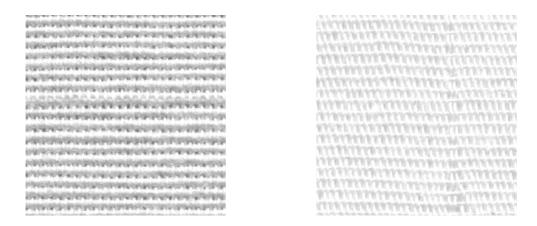
Figure 4.27: Double-pick and double-end
