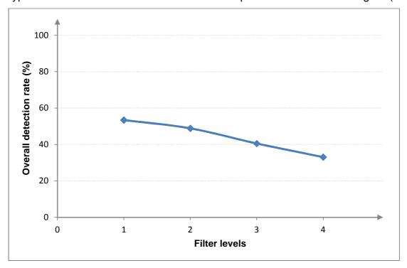
Figure 5.10 Effect of filter levels on the overall detection of simulated fabric
