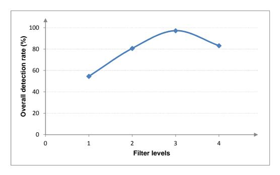
Figure 5.20: Effect of filter levels on the overall detection of real fabric
