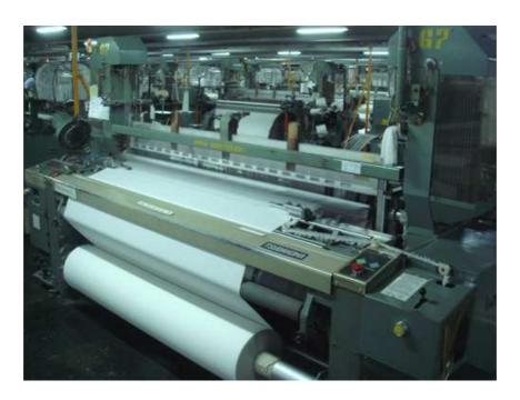
Figure 2.1: Modern (air-jet) looms
