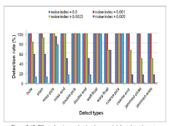
Figure 5.17: Effect of various noise levels on real defect detection rate
