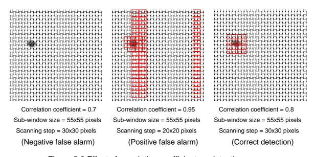
Figure 5.6 Effect of correlation coefficient on detection errors
