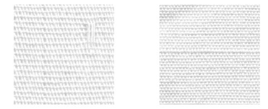
Figure 4.28: Warp-float and coarse-pick
