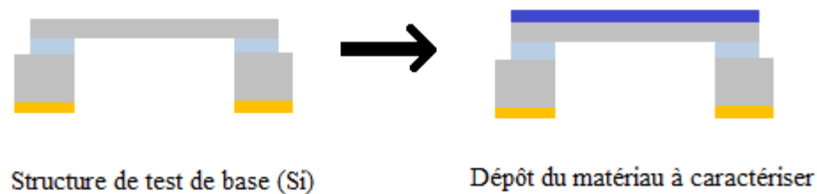
Figure 5.3-1. Structure de test bicouche
