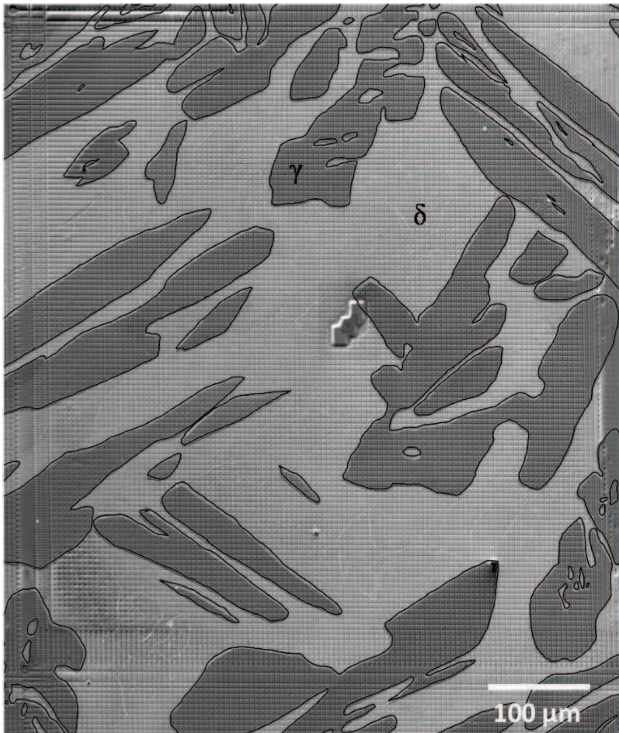
Figure C. 2. High resolution SEM micrograph of the D1_W microstructure (map2) in the undeformed configuration; sample iii. The compression will be applied vertically.
