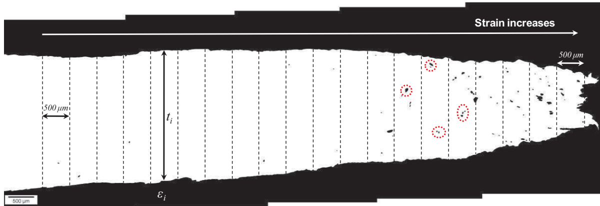
Figure III.8. Section perpendicular to the ligament in order to quantify the density of cracks per unit area (mm 2 ) as a function of strain; the dotted lines correspond to the 500 \mu m-step partition; the black arrow shows the position where the thickness was measured to estimate the strain; and the red circled zones highlight a few voids.
