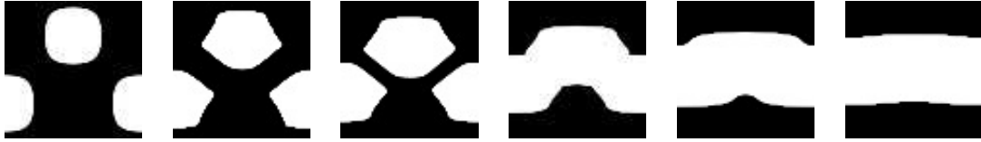
Figure 3.9: Optimization of the flexural stiffness with respect to the matter distribution in a square unit cell (iterations 1, 10, 20, 30, 40 and 50). The resulting shape is not interesting because global bending stiffness is zero. The shear stiffness must be also included into a multi-functional objective function.
