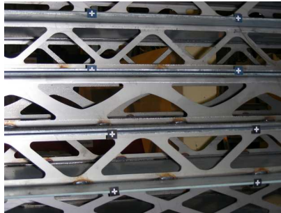
Figure 4.28: Sandwich samples with optimized and standard stiffeners.
