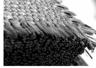
(c) Interlock fabric preform made of carbon fibres destined to be filled with a polymer matrix by RTM process (De Luycker et al., 2009).
