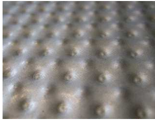
Figure 2.23: Example of embossed steel sheet made by ArcelorMittal.
