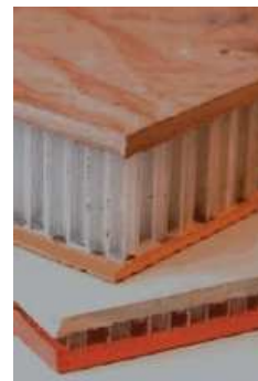
(b) Association of polymer honeycomb Nidaplast with a fiber reinforced concrete Ductal.
