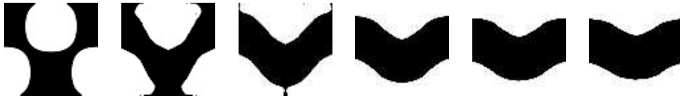
Figure 3.10: Optimization with area fraction \bar{A}_f = 0.5 and satisfying the constraint from the first iteration. Weighting factor is \alpha = 0.6 and pictures correspond to iterations 1, 10, 20, 30, 40 and 50.
