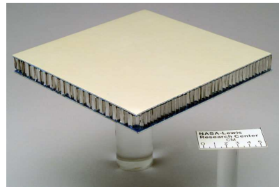
(b) Nasa development of sandwich with glass fibers reinforced polymer faces and a honeycomb polymer core.
