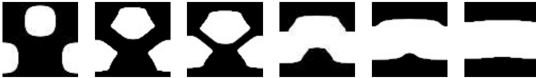
Figure 3.9: Optimization of the flexural stiffness with respect to the matter distribution in a square unit cell (iterations 1, 10, 20, 30, 40 and 50). The resulting shape is not interesting because global bending stiffness is zero. The shear stiffness must be also included into a multi-functional objective function.
