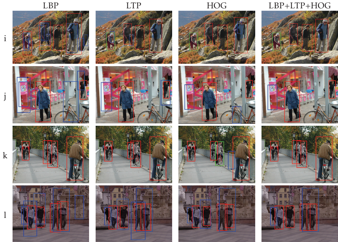
Figure 6.4: Some examples of detections from our latent single root detectors on the INRIA Person test set, for various feature sets. The red boxes indicate true detections according to the PASCAL VOC criteria, the blue boxes indicate false positives, and the green boxes indicate the ground truth annotations. Notice the similarity of the responses from HOG and LTP (although LTP is able to detect some instances missed by HOG – rows f, g, k), and the fact that the combined feature set significantly improves the results.
