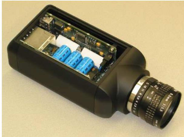
FIGURE 1.1 – La camera Philips inca
