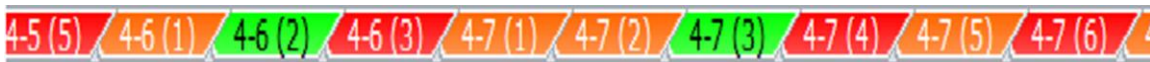
Figure 4-33. Staining tab code color following the readiness of the deliverable. Each tab represents the deliverable of a certain process with its rank. For example 4-6 (1) is the first output deliverable of the subprocess 4-6 (clause 6 of part 4 of ISO26262)
