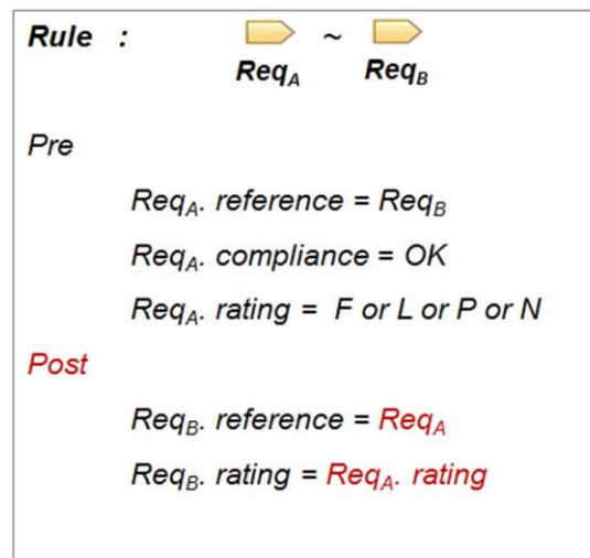
Figure 4-30. Assessment rule when two requirements in the different standards or completely compliant
