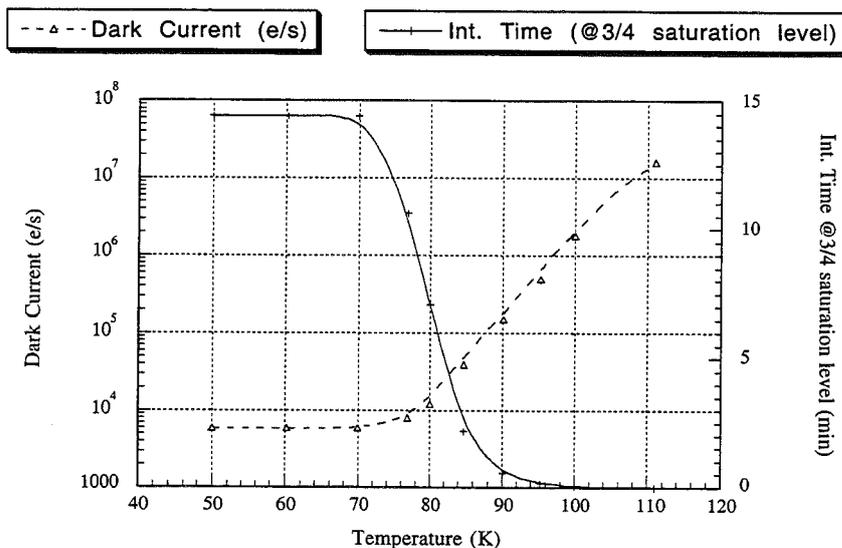
Figure 7: Dark current and integration time at 3/4 of the saturation level as a function of the temperature.
