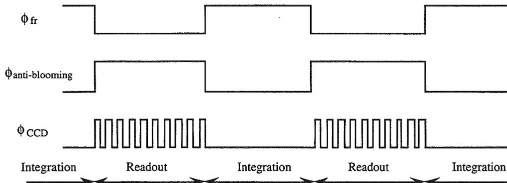
Figure 2 : Command clocks of the IRCCD in the "separated integration and readout phases" operating mode . The frame signal  $\Phi_{fr}$  is kept high during the integration phase and connects the photovoltaic level to the CCD and the integration capacitances. Then  $\Phi_{fr}$  goes to low level during the readout period while the anti-blooming signal is high and resets the charges to prepare the next integration. During the integration period, the CCD clocks  $\Phi_{CCD}$  are stopped.
