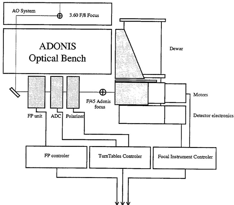
FIG. 2.—Scheme of the COMIC camera, its associated external units, and controllers
