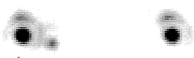
FIG. 13.—First COMIC  $L$ -band (3.5 μm) image of a PMS binary (*left*) together with its associated PSF reference star (*right*). The binary separation is 0".5, and the FWHM is 0".24 (diffraction limit).
