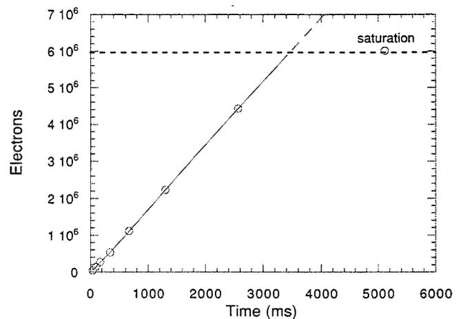
FIG. 10.—Linearity vs. integration time. The saturation level is reached above 6 × 10<sup>6</sup> electrons.
