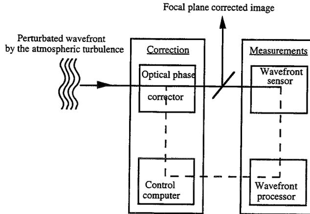
Figure 1 : Principle of the adaptive optics loop <sup>2</sup>
