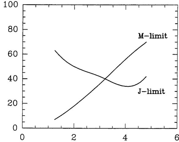
Figure 4: Quantum Efficiency as a function of  $\lambda$  for both optics (J limit & M limit). The two plots cross at  $\lambda \approx 3 \mu\text{m}$  where both objectives are outside their optimisation domain.
