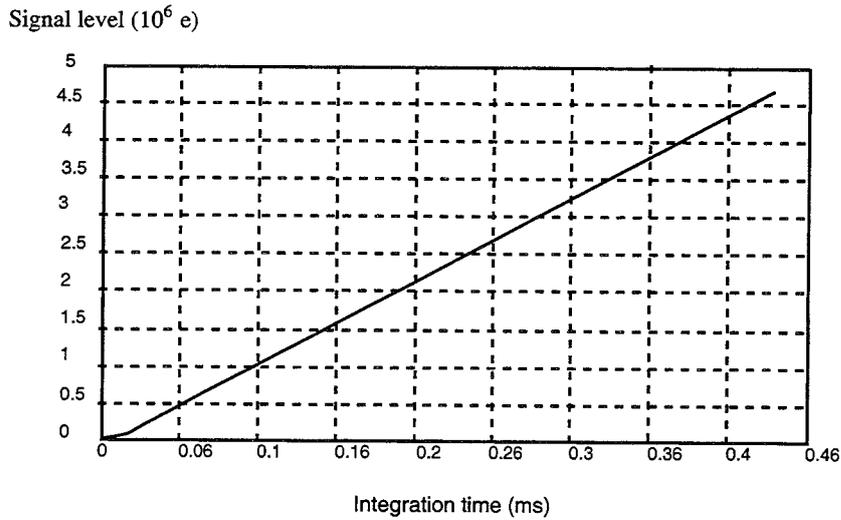
Figure 3: Detector linearity for a typical pixel.
