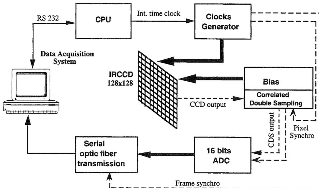
Figure 8 : Synoptic diagram of the control electronics.
